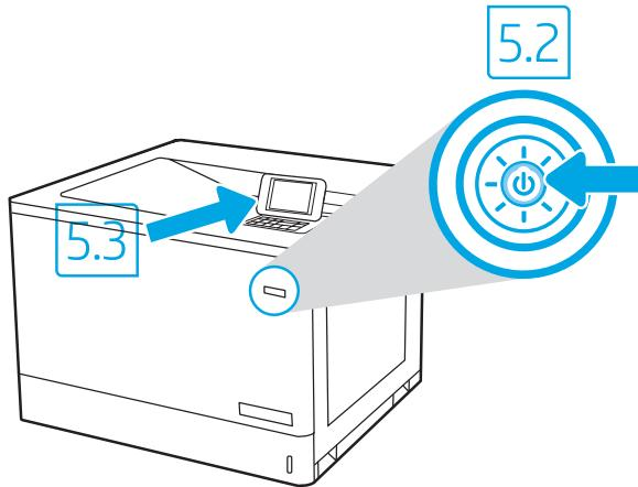
**EN** **5.1** Connect the power cable between the printer and a grounded AC outlet. **5.2** Turn on the printer. **5.3** On the **Initial Setup** screen, set the language, the location, the date/time format, and other features.
