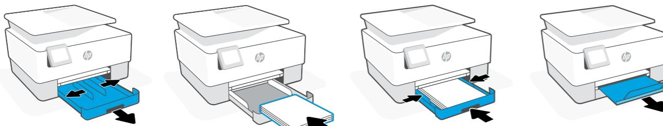
**EN** Open the paper tray and slide out the guides. Load Letter or A4 paper and adjust the guides. Close the tray. Pull open the output tray extender.
