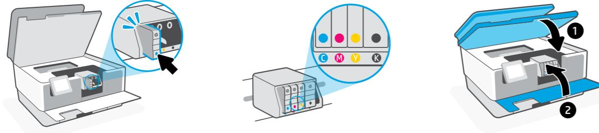
**EN** Insert each cartridge securely into the indicated slot. Close both doors.
