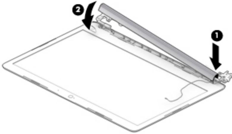
6. If it is necessary to replace the display hinges:
