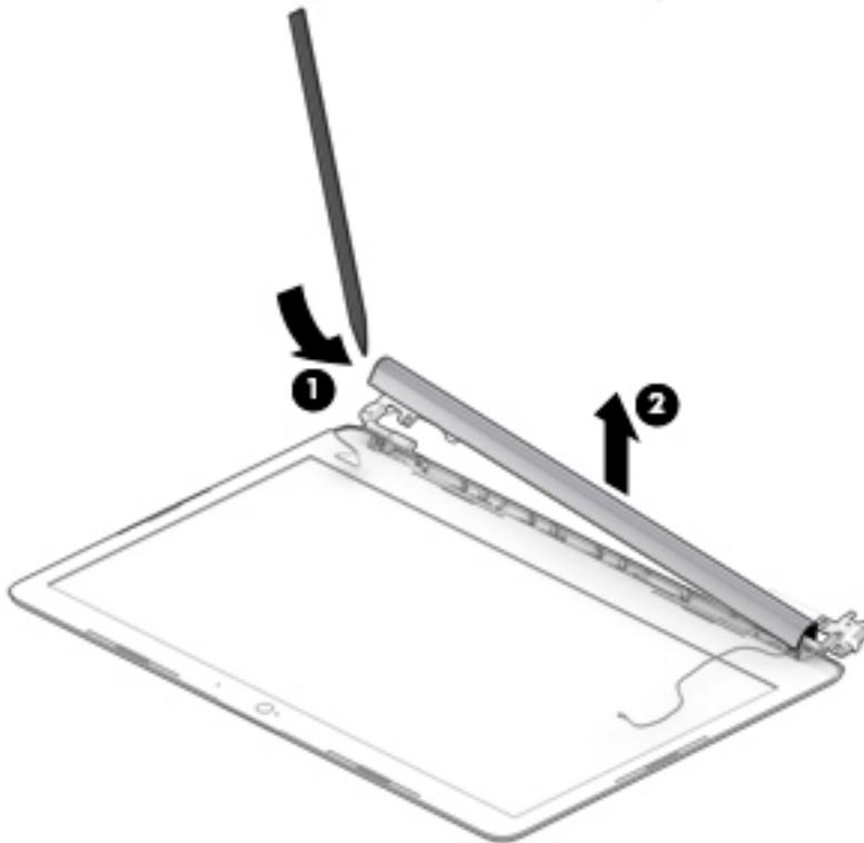
5. When replacing the hinge cover, make sure the hinges rotate downward as far as they can go. Align the cover **(1)**, and then start from above and rotate the cover downward onto the hinges **(2)**. Make sure the clips snap into place along the bottom of the display cover.
