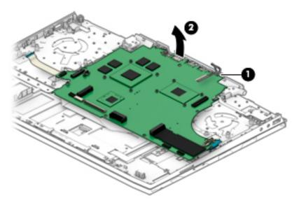
4. Release the USB cable (1), and then disconnect the audio board cable (2) from the bottom of the system board.
