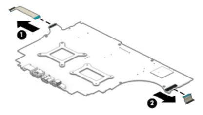
Reverse this procedure to install the system board.
