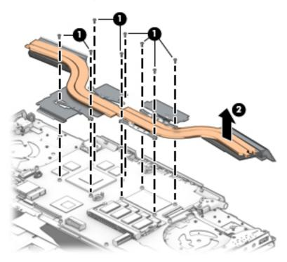
NOTE: The thermal material must be thoroughly cleaned from the surfaces of the heat sink and the system board components each time the heat sink is removed. Thermal paste is used on the processor (1) and (3) and the heat sink section (2) and (4) that services it.
