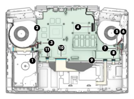
Remove the plastic guides (1) and M2.5x4 Phillips head screws (2). 2.
