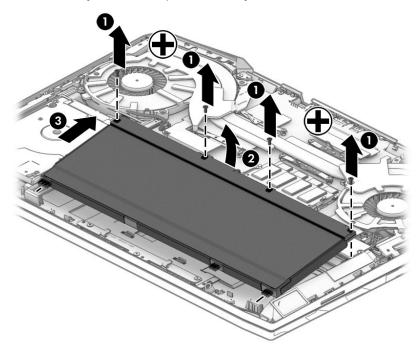
Reverse this procedure to install the battery.
