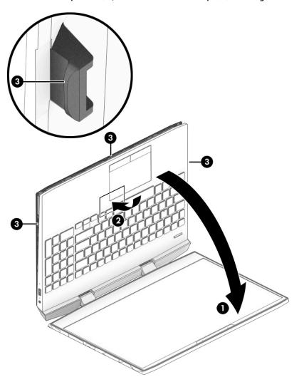
6. Shake the left and right sides (1) to release the base enclosure, and then lift the base enclosure (2) to remove it.
