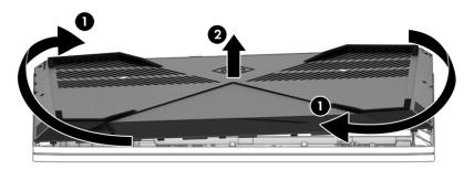
Reverse the removal procedures to install the base enclosure.
