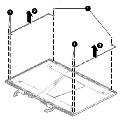
12. If it is necessary to replace the display hinge brackets, remove the six Phillips screws (1) that secure each bracket, and then remove the bracket (2) from the display enclosure.
