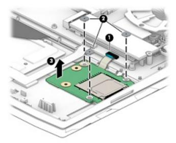
Reverse this procedure to install the smart card reader.
