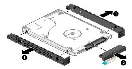
Reverse this procedure to install the hard drive.
