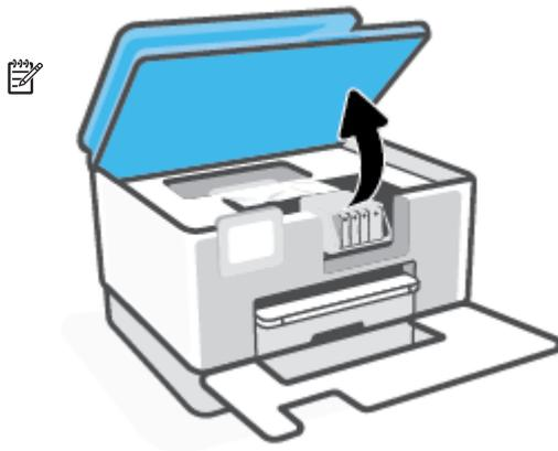
4. Press the front of the cartridge to release it, and then remove it from the slot.
