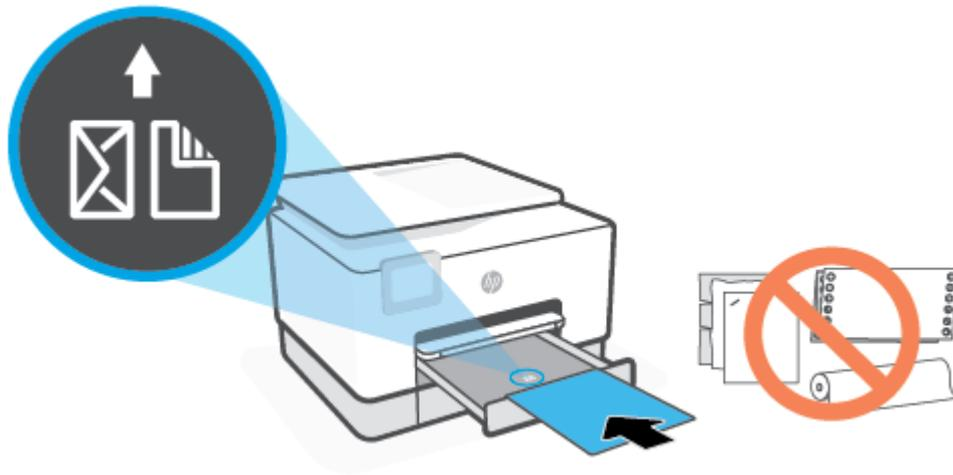
Make sure the stack of paper is aligned with the appropriate paper size lines on the front of the tray. Also, make sure the stack of paper does not exceed the stack height marking on the left edge of the tray.
