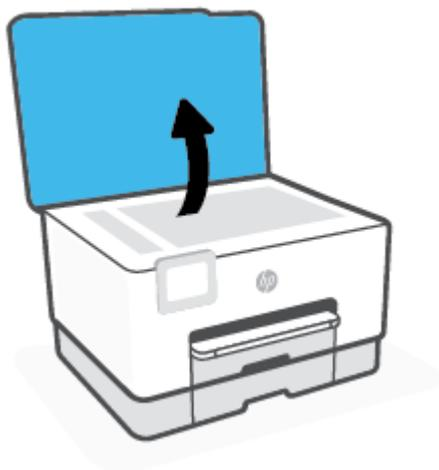
2. Clean the scanner glass and lid backing by using a soft, lint-free cloth that has been sprayed with a mild glass cleaner.
