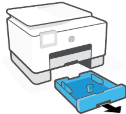
2. Press the button on the paper-length guide and slide the guide at the same time towards the edge of the tray as far as possible.
