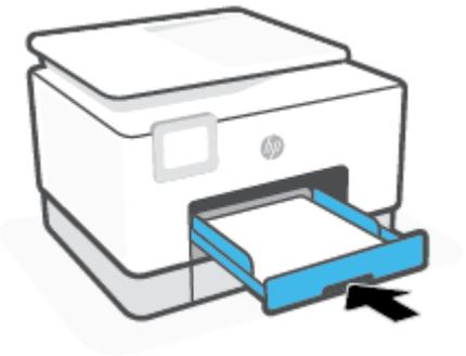
5. Insert the output tray back into the printer.
