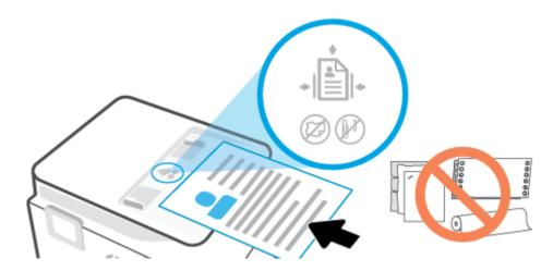
Slide the paper-width guides inward until they stop at the left and right edges of the paper.
