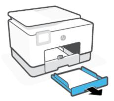
3. Check the gap in the printer where the input tray was. Reach into the gap and remove the jammed paper.
