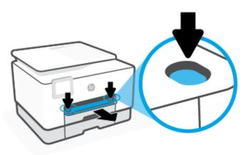
2. Pull Tray 2 out of the printer completely.
