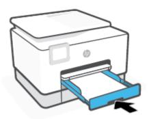
**NOTE:** When you insert the input tray, the input tray extension remains outside of the printer. This is the expected result.
