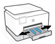
3. Press the button near the front left of the tray to extend the input tray.
