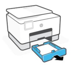
Check the gap in the printer where the input tray was. Reach into the gap and remove the jammed paper.
