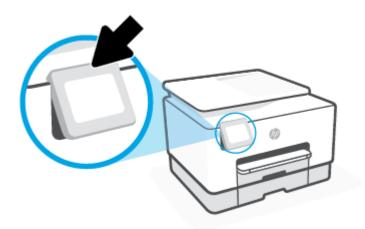
**NOTE:** Return the control panel to its original position by pushing down the bottom until it is back in place.
