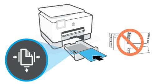
Make sure the stack of paper is aligned with the appropriate paper size lines on the front of the tray. Also, make sure the stack of paper does not exceed the stack height marking on the left edge of the tray.
