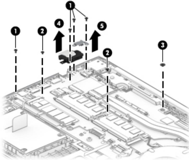
7. Rotate the right side of the system board upward **(1)**.
