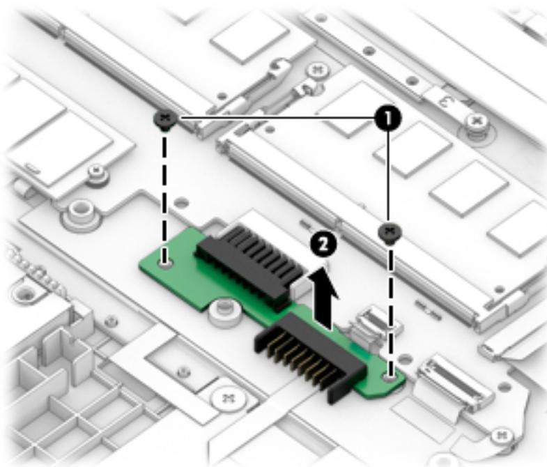
Reverse this procedure to install the battery connector board.
