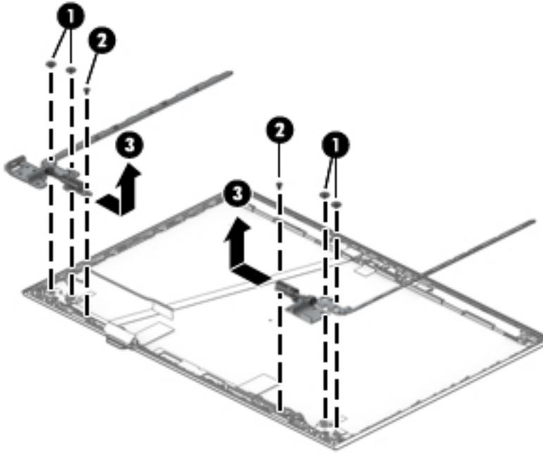
13. If it is necessary to replace the WLAN antennas, peel the antennas from the enclosure (1), remove the cables from the clips in the bottom of the enclosure (2), and then remove the antennas and cables from the enclosure (3).
