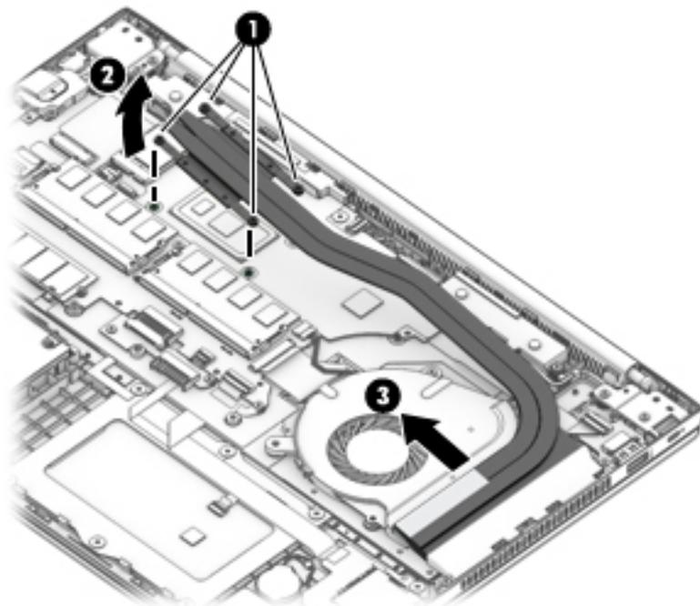
3. Thoroughly clean thermal material from the surfaces of the system board component **(1)** and the heat sink **(2)** each time you remove the heat sink. All heat sink and system board spare part kits include thermal material.
