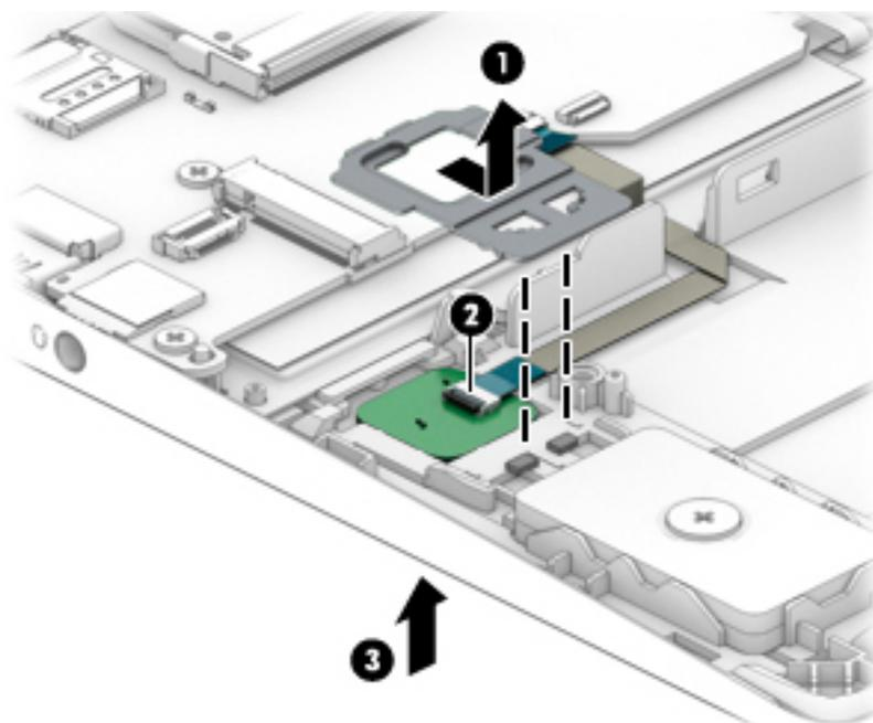
Reverse this procedure to install the fingerprint sensor assembly.
