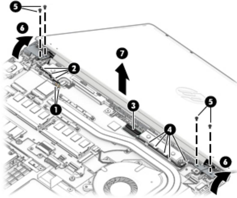
11. If it is necessary to remove the hinges from the display enclosure, remove the two Phillips broad head M2.5 × 2.5 screws **(1)** and the Phillips M2.0 × 4.0 screw **(2)** from the bottom of each hinge.
