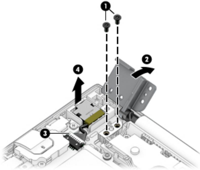
Reverse this procedure to install the power connector cable.
