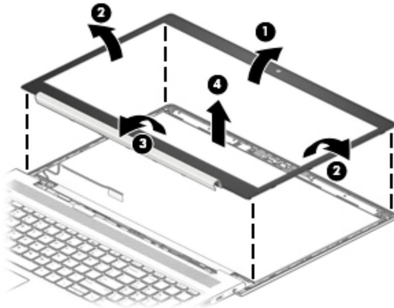
3. If it is necessary to remove or replace the display panel, use a tweezer to grasp the end of the two pieces of tape that secure the bezel to the display enclosure **(1)**. The tape is positioned under the left and right sides of the display panel.
