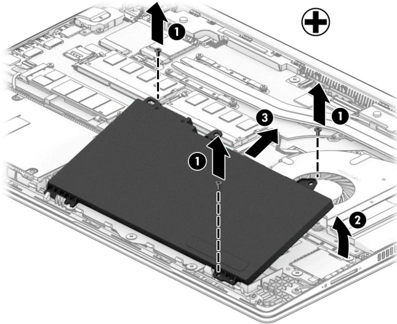
Reverse this procedure to install the battery.
