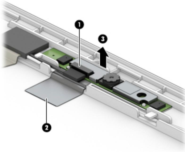
9. If it is necessary to remove or replace the IR camera, disconnect the cable from both sides of the camera (1), and then peel the camera module up to remove it from the adhesive that secures it to the enclosure (2).
