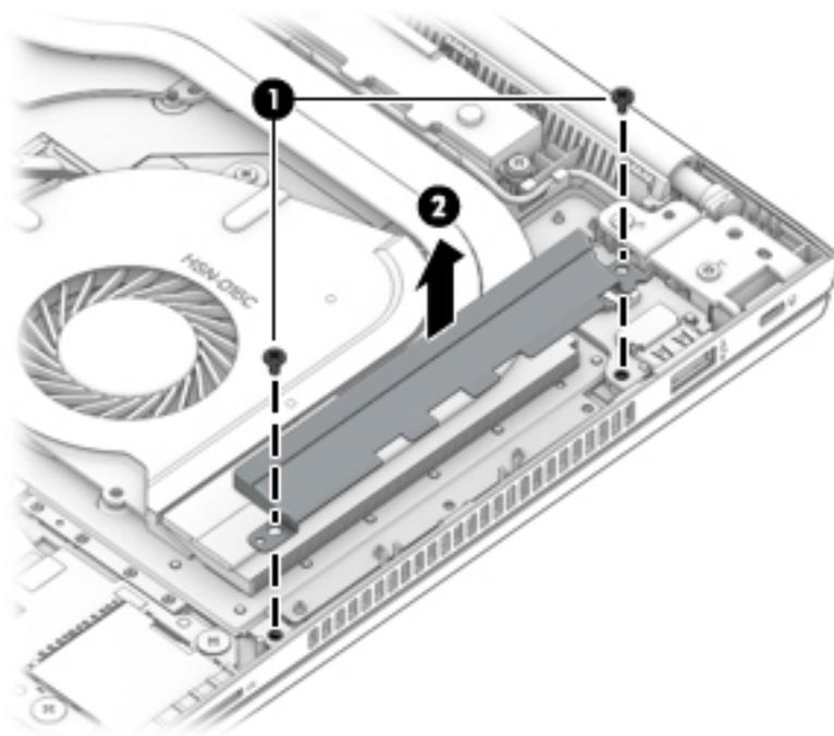
3. Disconnect the cable from the ZIF connector on the power/USB board **(1)**.
