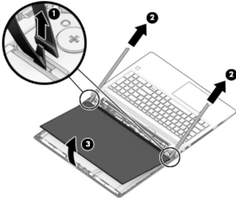
6. Lift the tape from atop the connector on the display panel **(1)**, lift the locking latch **(2)**, and then disconnect the cable from the panel **(3)**.
