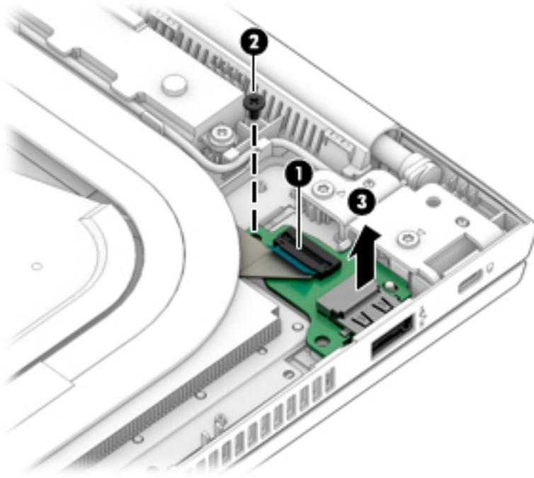
Reverse this procedure to install the power/USB board.
