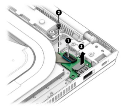
Reverse this procedure to install the power/USB board.
