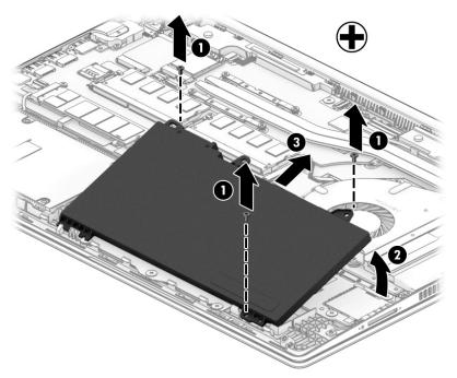
Reverse this procedure to install the battery.
