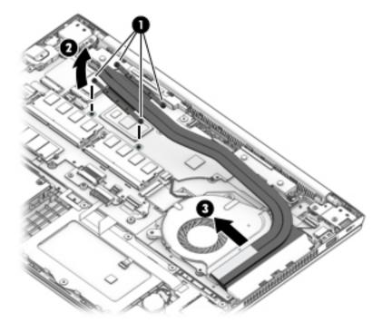
Thoroughly clean thermal material from the surfaces of the system board component (1) and the heat sink (2) each time you remove the heat sink. All heat sink and system board spare part kits include thermal material.
