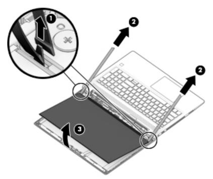
**6.** Lift the tape from atop the connector on the display panel **(1)**, lift the locking latch **(2)**, and then disconnect the cable from the panel **(3)**.
