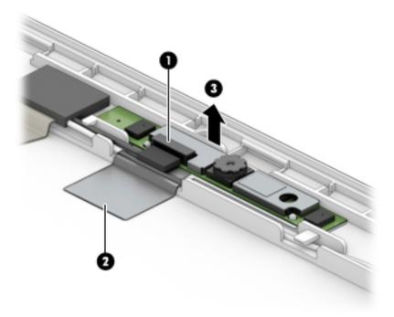
If it is necessary to remove or replace the IR camera, disconnect the cable from both sides of the camera
