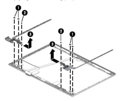
**13.** If it is necessary to replace the WLAN antennas, peel the antennas from the enclosure **(1)**, remove the cables from the clips in the bottom of the enclosure **(2)**, and then remove the antennas and cables from the enclosure **(3)**.
