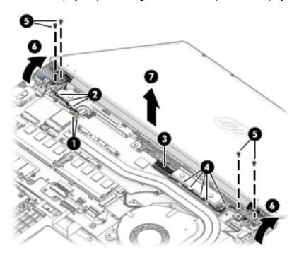
11. If it is necessary to remove the hinges from the display enclosure, remove the two Phillips broad head M2.5 × 2.5 screws (1) and the Phillips M2.0 × 4.0 screw (2) from the bottom of each hinge.
