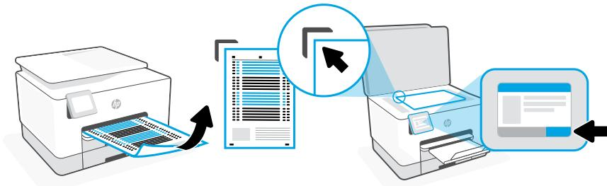
**EN** Use the control panel to print and scan the alignment page.
