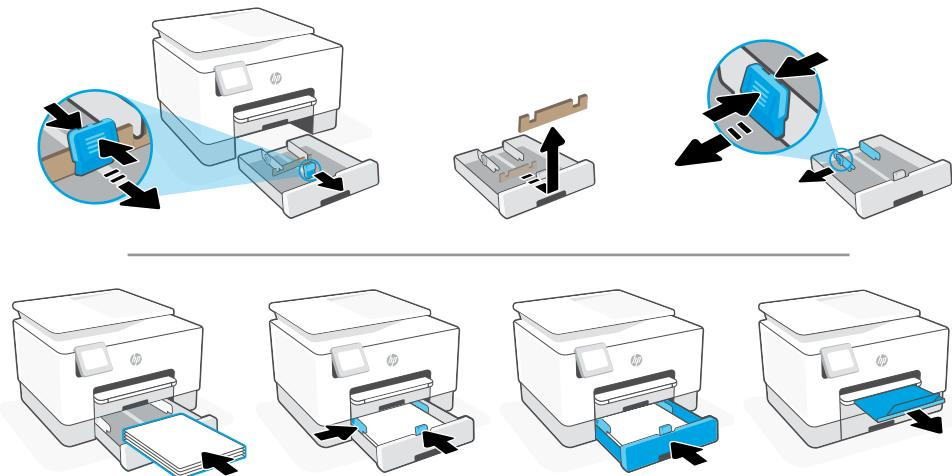
**EN** Open the paper tray. Slide out the front length-guide, remove the cardboard, and slide out the width-guides. Load Letter or A4 paper and adjust the guides. Close the tray and pull open the output tray extender.
