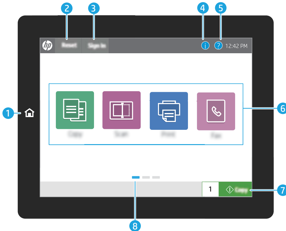
Gambar 1-6 Tampilan panel kontrol 8 inci (E77428dn, E77422dn)
