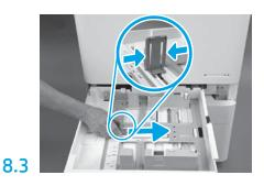
Squeeze the sides of the tab, and then slide to adjust the paper width.
