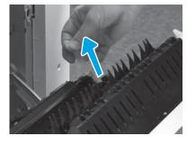
Carefully remove the strapping tape at the rear of the transfer unit.
