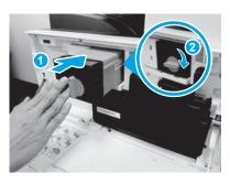
Align the toner cartridge with its slot, insert the toner cartridge into the printer (callout 1). And then, lock the latch (callout 2).
