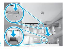
Push down on the blue tab in the back of the tray. At the same time, pinch or squeeze the blue tab in the front of the tray and slide to adjust to the proper paper length. Both tabs are spring-loaded and will lock, once released.
