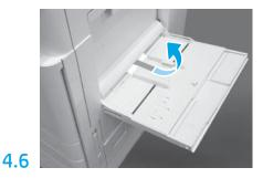
Open Tray 1 on the right side of the printer, and then remove the foam near the pickup roller.
