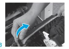
Carefully remove the strapping tape at the front of the transfer unit.
