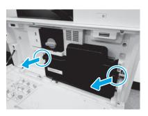
Push the latches on each side of the TCU and then remove the TCU.
