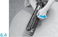
Pull straight out to remove the orange charge roller shipping lock.
