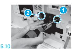
Push and hold the imaging unit in place while installing the first screw (callout 1) to secure the imaging unit. Install the second screw (callout 2).
