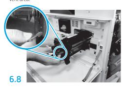
Hold the imaging unit with one hand on the bottom and the other hand on the gray handle at the front.
