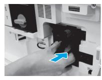
Slide the imaging unit into the device.
