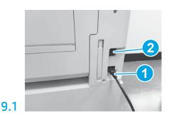
Connect the power cord to the printer and the wall receptacle (callout 1).
