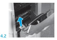
Open the right door and then remove the shipping label directing you to the transfer area.
