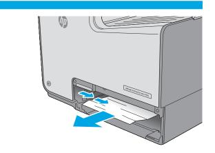
Remove any jammed paper from the feed rollers inside the printer. First pull the paper to the right, and then pull it forward to remove it.
