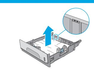
Remove any jammed or damaged sheets of paper. Verify that the tray is not overfilled and that the paper guides are adjusted correctly.
