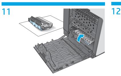
Lift the green tab to return the platen to the operating position.
