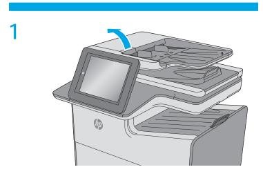
Lift the latch to release the document-feeder cover.
