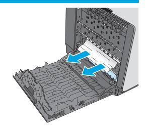
Gently pull out any jammed paper from the rollers and delivery area. If the paper tears, make sure to remove all remnants.
