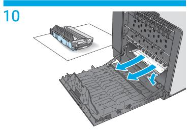
Lower the platen by pressing down on the green tab. This will cause the printer to try to feed the sheet through the print zone. You might need to gently pull on the sheet if it does not feed. Remove the sheet.
