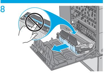
Remove the ink-collection unit by pulling it out with both hands. Set the unit aside, upright, on a piece of paper to prevent spills. **CAUTION:** When removing the ink-collection unit, avoid making direct contact with the black cylinder to prevent pigment smear on skin or clothes.
