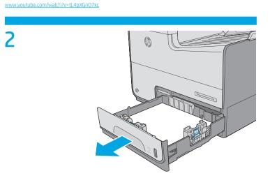
Pull Tray 2 completely out of the printer by pulling and lifting up slightly.
