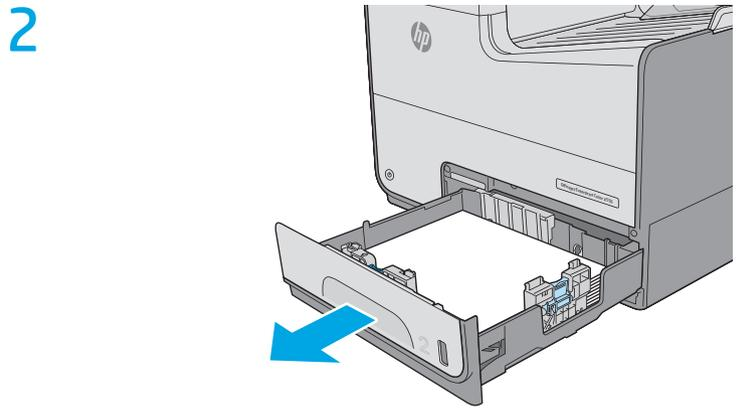
Pull Tray 2 completely out of the printer by pulling and lifting up slightly.
