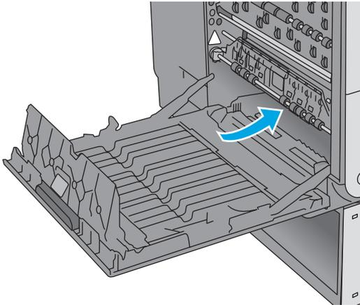
After removing the ink-collection unit, look deep inside the area where it was located and remove any paper or debris found.
