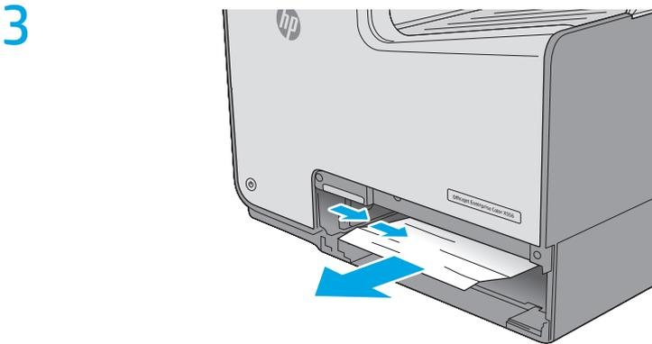
Remove any jammed paper from the feed rollers inside the printer. First pull the paper to the right, and then pull it forward to remove it.
