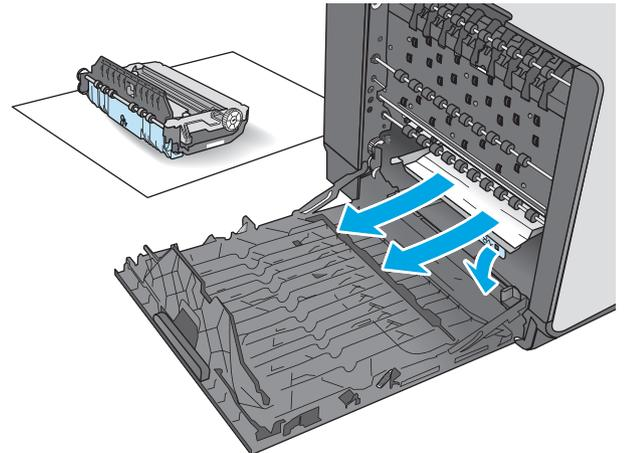
Lower the platen by pressing down on the green tab. This will cause the printer to try to feed the sheet through the print zone. You might need to gently pull on the sheet if it does not feed. Remove the sheet.
