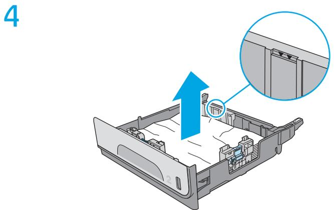
Remove any jammed or damaged sheets of paper. Verify that the tray is not overfilled and that the paper guides are adjusted correctly.
