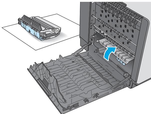
Lift the green tab to return the platen to the operating position.
