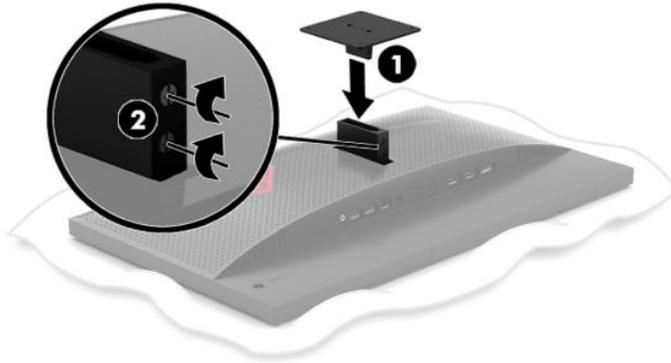
3. To attach the monitor head to a swing arm or other mounting device, insert four mounting screws through the holes on the mounting device and into the screw holes on the VESA mounting bracket.
