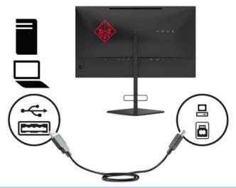
**NOTE:** You must connect the USB Type-B upstream cable from the source device (computer, laptop, gaming console) to the rear of the monitor to enable the USB Type-A downstream ports on the monitor. For more information, see <u>Connecting USB devices on page 7</u>.
