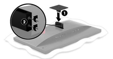
3. To attach the monitor head to a swing arm or other mounting device, insert four mounting screws through the holes on the mounting device and into the screw holes on the VESA mounting bracket.
