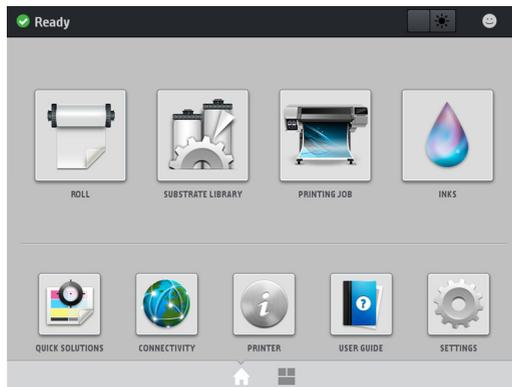
There is an alternative home screen that you can see by sliding your finger across the screen to the left or pressing the widget button in the bottom central area of the screen. It summarizes the status of the ink cartridges, the substrate, and the current print job.
