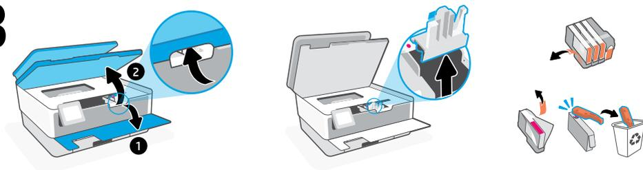
**EN** Open the front door and then lift the cartridge access door by the scanner lid. Remove the plastic guard. Remove cartridge packaging, tape, and orange guards.
