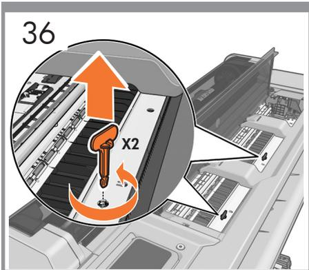
**IMPORTANT:** remove the 2 (T500 36" ONLY), or 1 (T500 24" ONLY) orange colored carriage locking pin(s).
