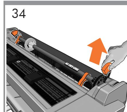
Remove the 2 spindle tapes and retainers.
