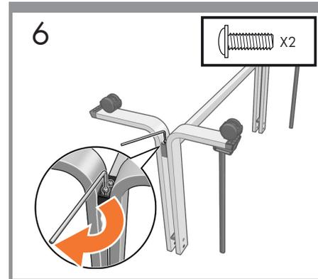
Fix into place with 2 screws.
