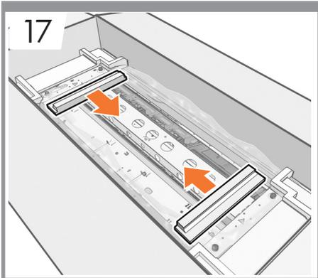
Remove the 2 (1 each side) end cap sections.
