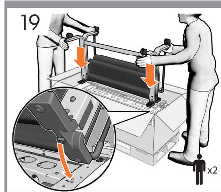
Fix the legs to the printer with 4 screws (2 each side). Note: leave the screws loose; don't fully tighten yet.
