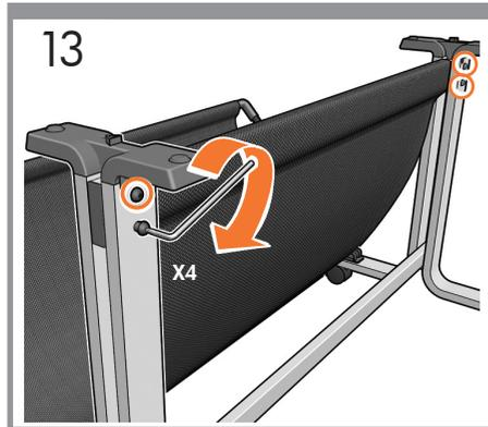
Fully tighten the 4 screws (2 each side).
