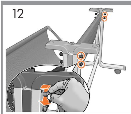
Tighten the 4 screws by hand (2 each side).
