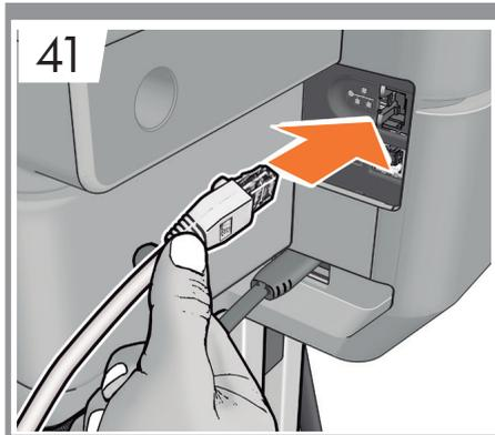
Connect the printer with the Ethernet cable if you plan to connect by LAN. If not: follow the instructions that come later in step 53.
