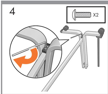
Fix into place with 2 screws.
