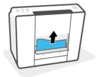
5. Close the cleanout door. Gently push the door towards the printer until both latches snap into place.
