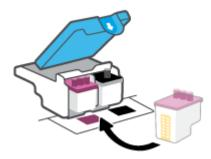
9. Close the printhead latch. Make sure the printhead latch is properly closed to avoid problems such as carriage jams.
