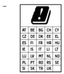
**CAUTION**: IEEE 802.11x wireless LAN with 5.15-5.35 GHz frequency band is restricted for **indoor use only** for all countries reflected in the matrix. Using this WLAN application outdoor might lead to interference issues with existing radio services.
