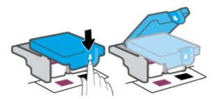
d. Remove the printhead from the carriage.
