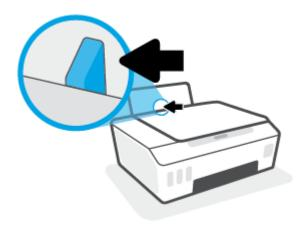
3. Insert a stack of paper into the input tray with the short edge down and the print-side up, and slide the stack of paper down until it stops.
