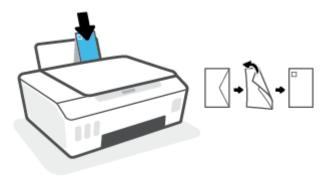
**b.** For envelope with the flap on the short edge, insert the envelope vertically with the flap on the top and facing down.
