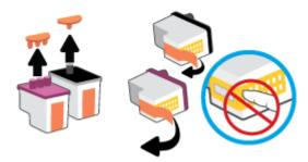
NOTE: Do not touch the electrical contacts on the printhead.
