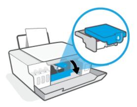
5. Push down to open the printhead latch.
