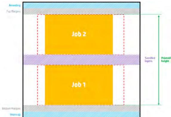
**Available printable height = Printable height – (Job CAD height + Sacrifice layers)**
