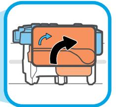
EN Open doors. Wait for carriage to move to center and stop. Turn orange handle.
