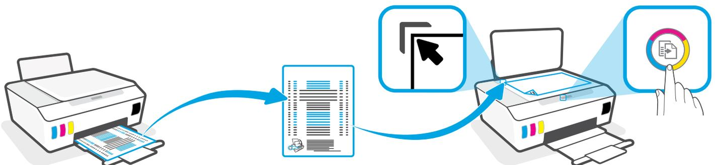
EN Scan the alignment page printed by pressing
