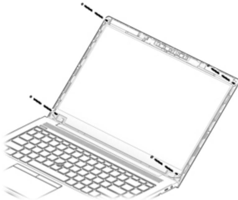
14. Rotate the display panel over onto the keyboard **(1)**.
