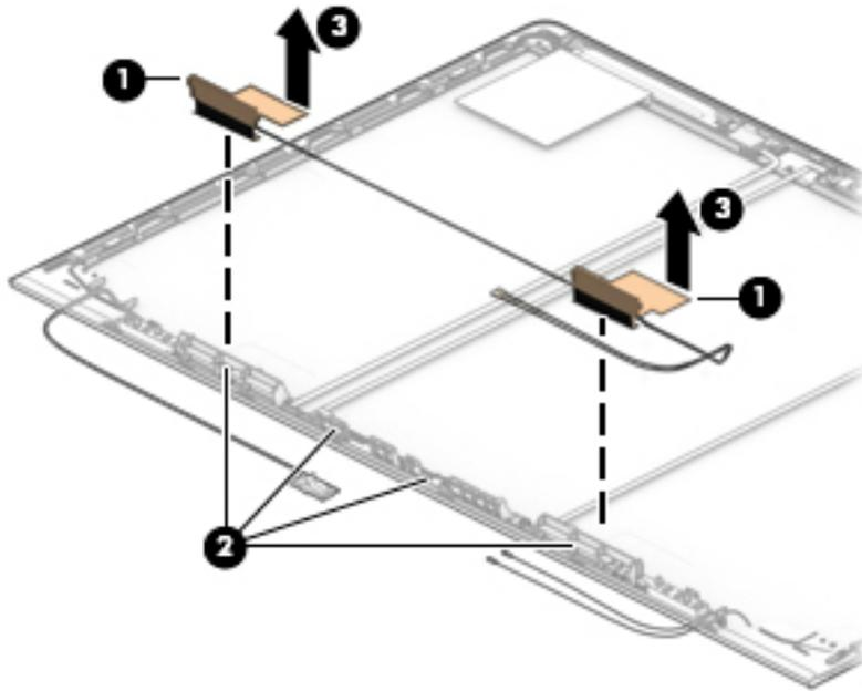
20. If it is necessary to replace the WWAN antenna cables, peel the antennas from the top of the display enclosure (1), remove the antenna cables from the bottom and sides of the display enclosure (2), and then remove the antenna cables (3).
