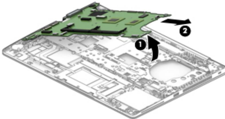
Reverse this procedure to install the system board.
