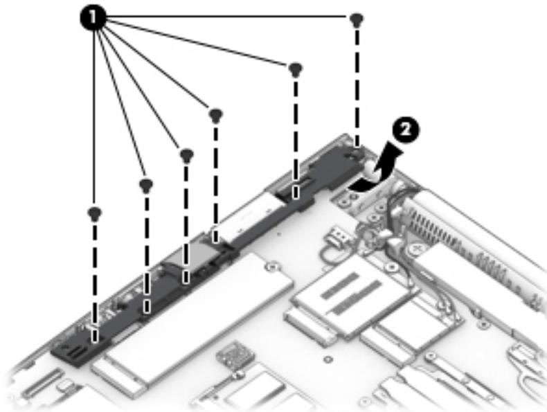
Reverse this procedure to install the RJ-45 assembly.
