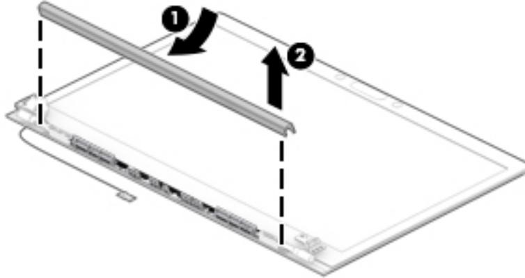
The display hinge cover for touch displays is available in the Hinge Kit as spare part number L15538-001. The display hinge cover for non-touch displays is available in the Hinge Kit as spare part number L15539-001.
