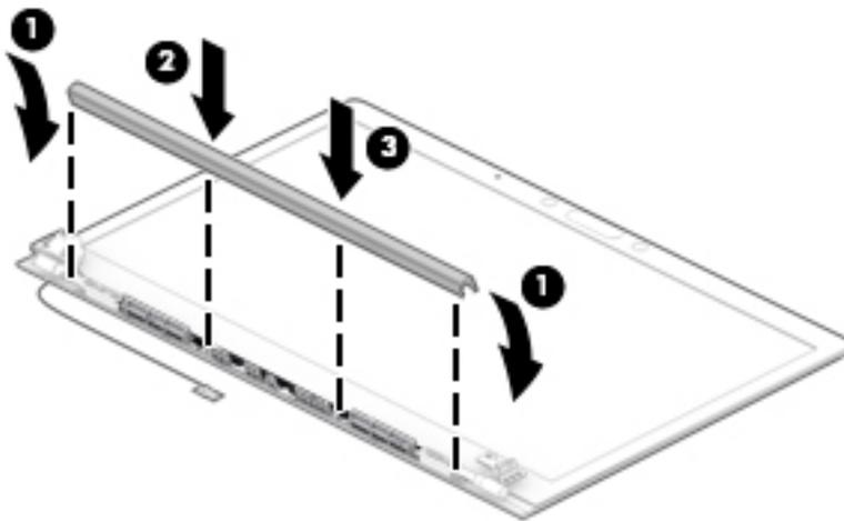
9. To remove the display bezel, flex the top **(1)** of the bezel, the inside edges of the left and right sides **(2)**, and then the bottom **(3)** of the bezel until it releases from the display enclosure.
