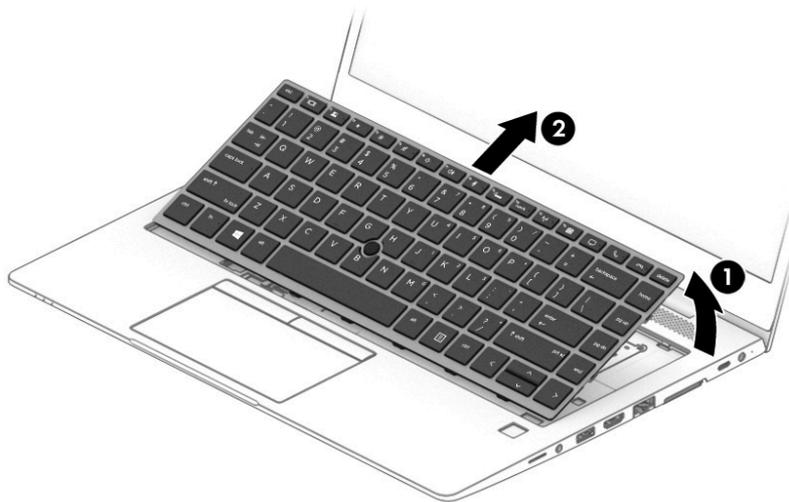
5. Rotate the keyboard over onto the palm rest **(1)**.
