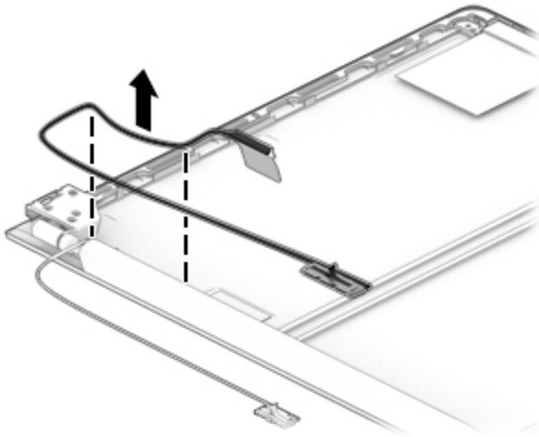
18. If it is necessary to replace the camera/ambient light sensor cable:
