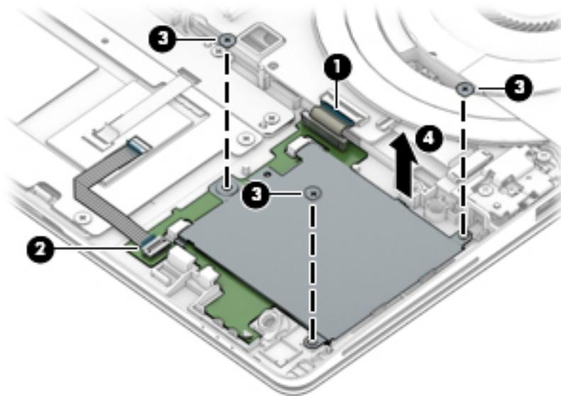
Reverse this procedure to install the smart card reader.
