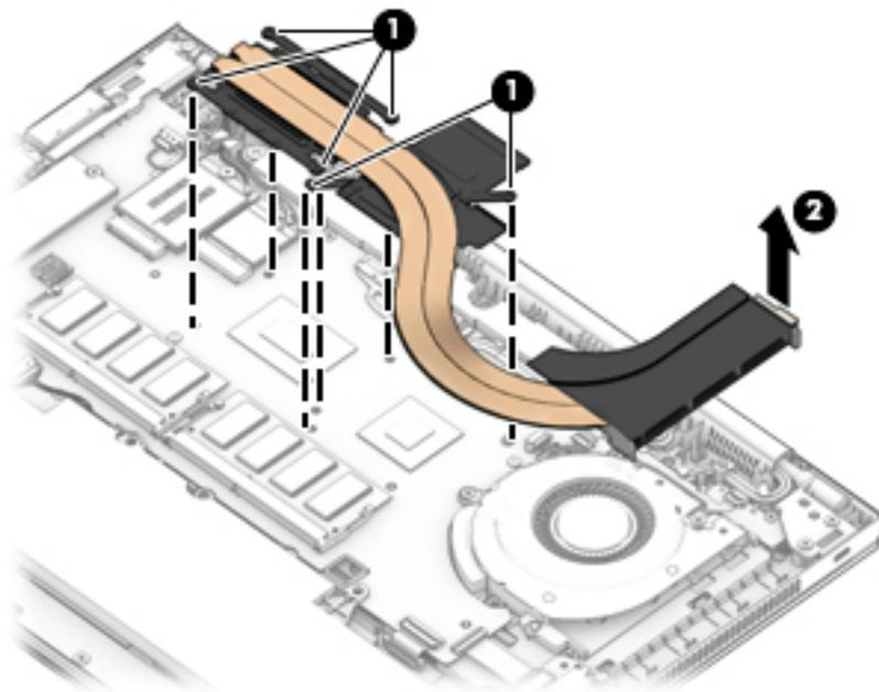
2. The heat sink and system board use both thermal grease and thermal pads. Thoroughly clean this thermal material each time the heat sink is removed. Replacement thermal material is included with the heat sink and system board spare part kits.
