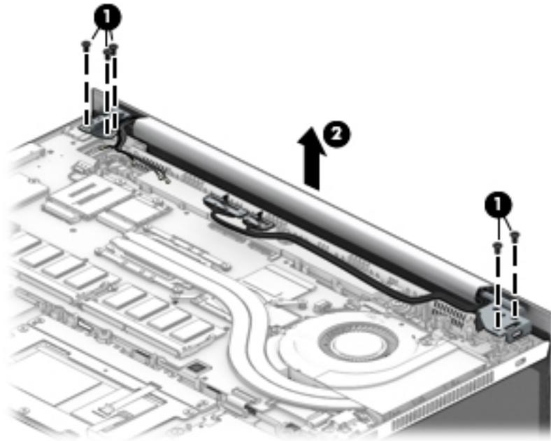
8. To remove the display hinge cover, rotate top of hinge cover away from display enclosure to release the tabs **(1)**, and then pull the cover off the enclosure **(2)**.
