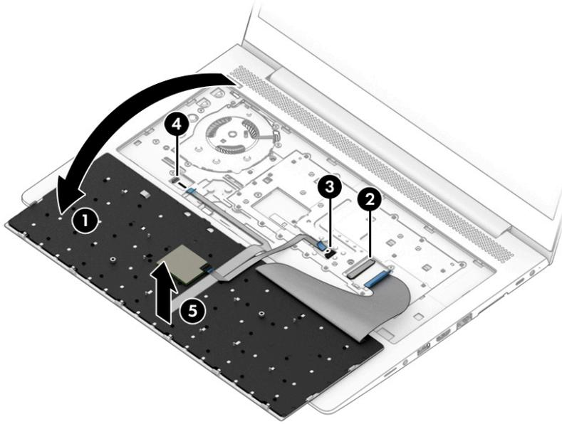
Reverse this procedure to install the keyboard.
