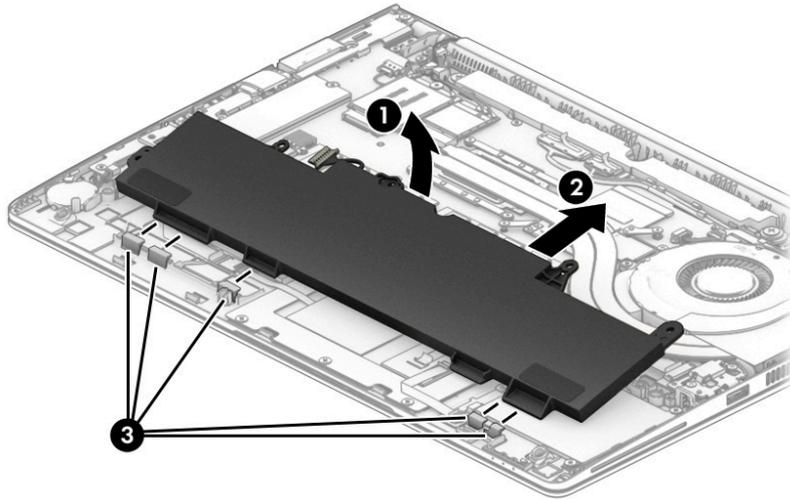
Reverse the removal procedures to install the battery.
