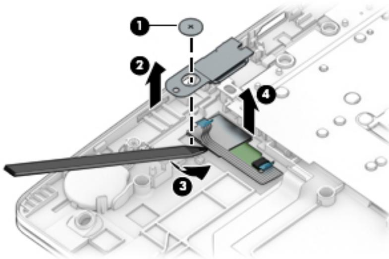
Reverse this procedure to install the fingerprint reader assembly.
