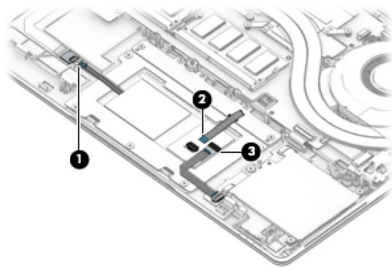
4. Remove the five Phillips M2.0 × 2.5 screws **(1)** that secure the touchpad to the computer.
