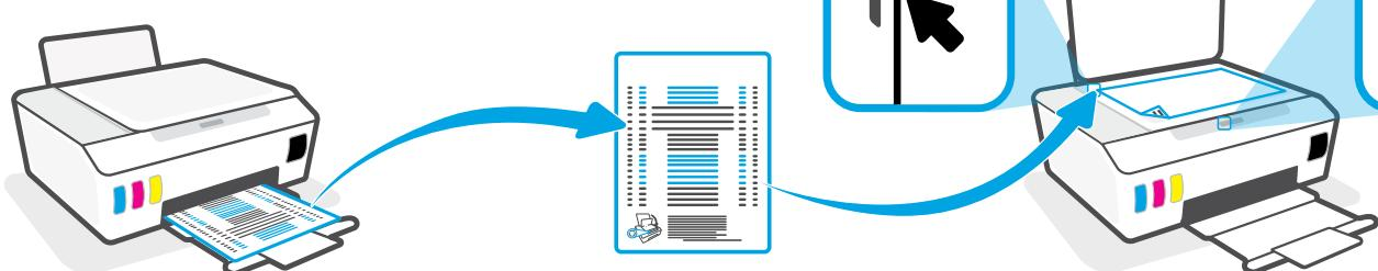
EN Scan the alignment page printed by pressing (Color Copy button).
