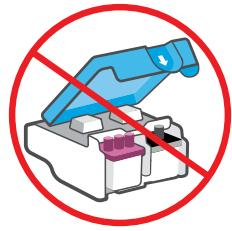
**EN** After setup, do not open blue latch unless instructed to do so.
