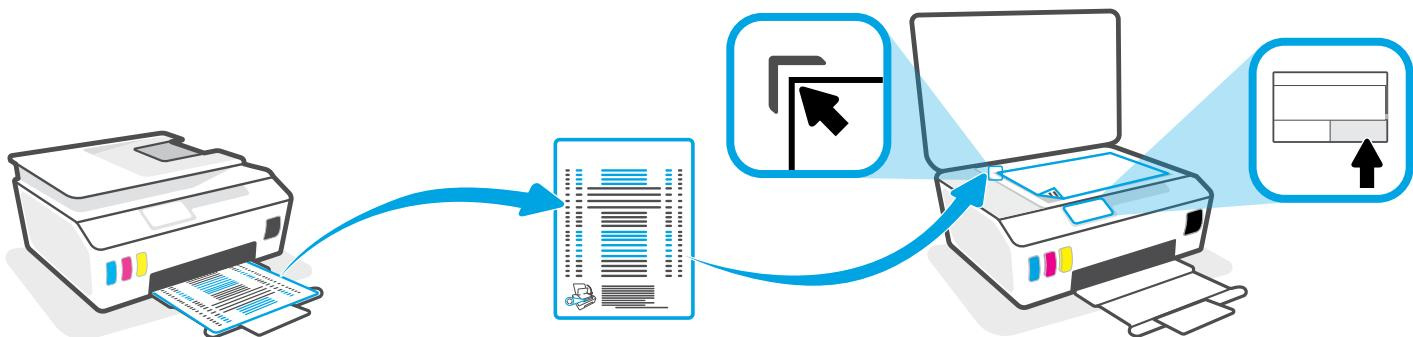
**EN** Scan the alignment page printed by following the on-screen instructions.
