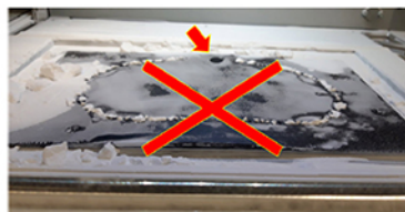
Platform installed incorrectly. Gap towards the rear
