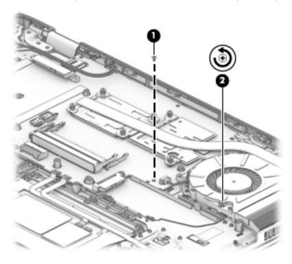
6. Lift the right side of the system board (1), and then pull it to the right to remove it from the computer (2).
