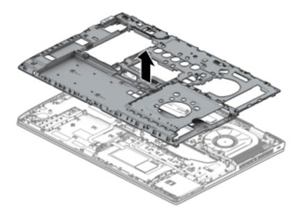
Reverse this procedure to install the internal frame.
