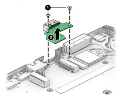
Reverse this procedure to replace the serial port board or VGA port board.
