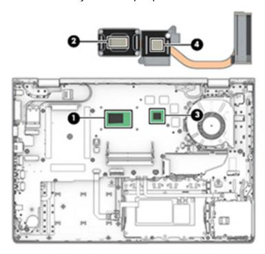
Reverse this procedure to install the heat sink assembly.
