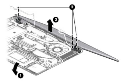
Remove the display assembly components:
