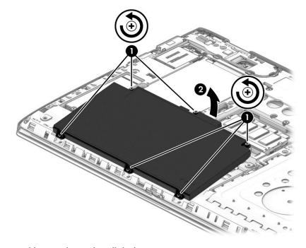
Reverse this procedure to install the battery.
