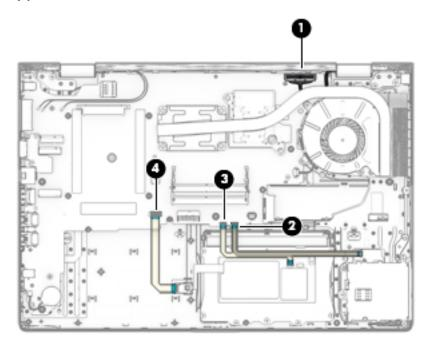
5. Remove the Phillips M2.0 × 2.5 screw (1), and then loosen captive Phillips screw (2) on the fan.
