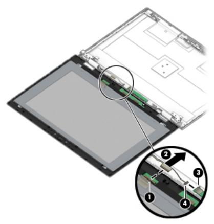
d. Remove the four Phillips M2.0 × 1.6 screws (1) that secure the display panel to the display cover. **e.** Lift the panel from the display cover **(2)**.
