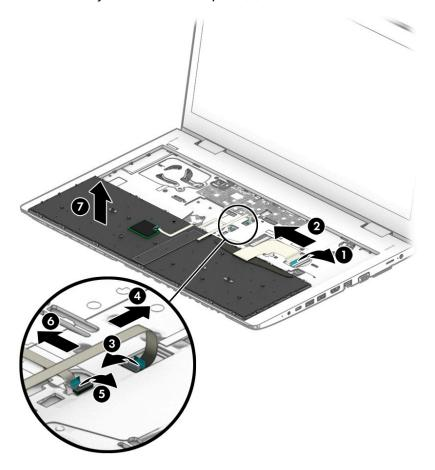
Reverse this procedure to install the keyboard.
