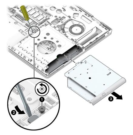
Reverse this procedure to install the optical drive.
