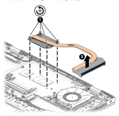
3. Thoroughly clean the thermal material from the surfaces of the system board components (1) and the heat sink (2) each time you remove the heat sink. Replacement thermal material is included with the heat sink and system board spare part kits.
