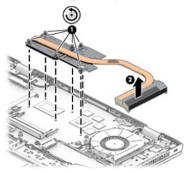
3. Thoroughly clean the thermal material from the surfaces of the system board components (1)(3) and the heat sink (2)(4) each time you remove the heat sink. Replacement thermal material is included with the heat sink and system board spare part kits.
