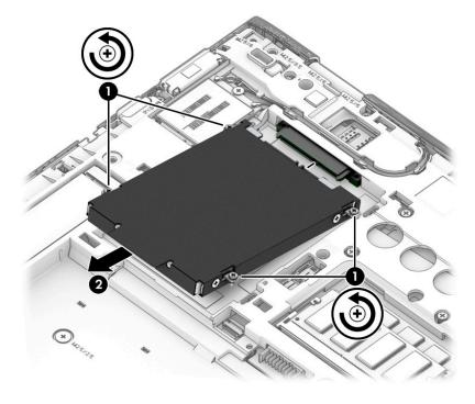
If it is necessary to disassemble the hard drive, remove the four Phillips M3.0  $\times$  3.0 screws (1), and then slide the drive out of the drive cover (2).
