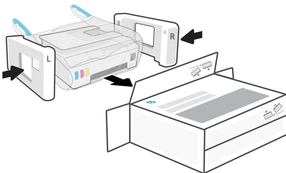
**EN** Repack the printer the way it was originally packed, and then reseal the box.
