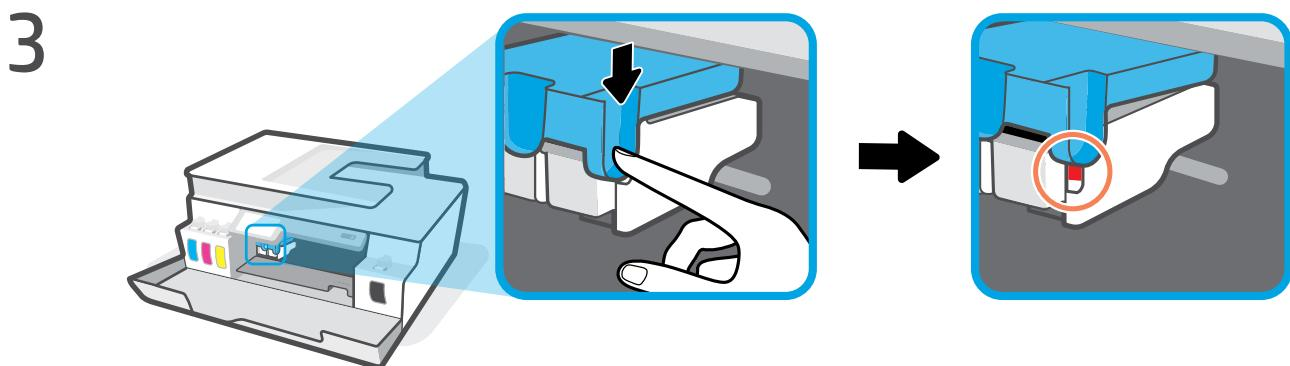
**EN** Press down on the side of the blue latch to open.
