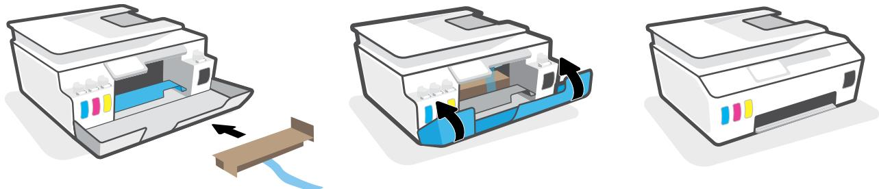
**EN** If repacking printer, reinsert cardboard restraint. Close doors.
