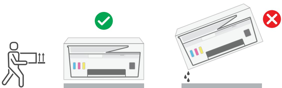
EN Keep printer upright and level to prevent ink leakage.
