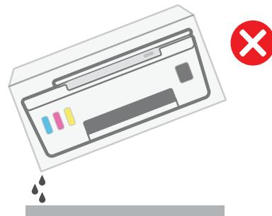
**EN** Keep printer upright and level to prevent ink leakage.
