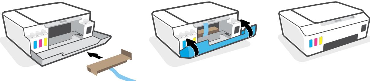
**EN** If repacking printer, reinsert cardboard restraint. Close doors.
