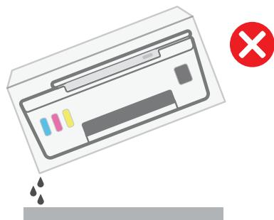
**EN** Keep printer upright and level to prevent ink leakage.
