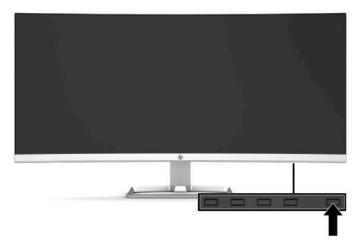
Press the power button on the monitor to turn it on.
