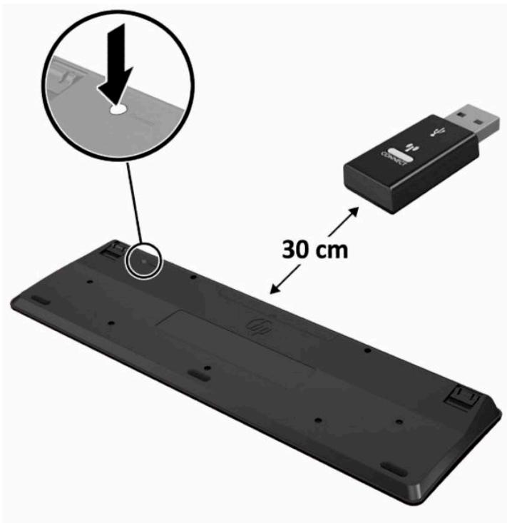
5. Press the Connect button on the receiver for approximately five seconds. The status light on the receiver will flash for approximately 30 seconds after the Connect button is pressed.
