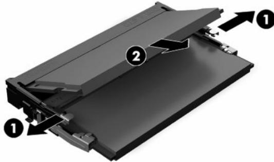
4. Slide the new memory module into the slot (1) at approximately a 30° angle, then press the memory module down (2) so that the latches lock it in place.
