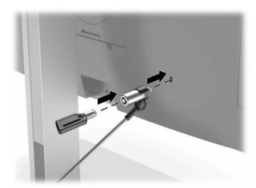
**IMPORTANT:** Use caution when adjusting the tilt, swivel, or height of the computer if a security cable is installed. The cable or the lock may interfere with the adjustment.
