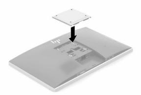
To attach the computer to a swing arm (sold separately), insert the four 20 mm screws that are supplied with the computer through the holes on the swing arm plate and into the mounting holes on the computer.
