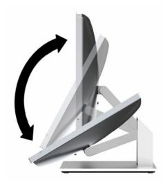
To adjust the computer position from an upright position to the reclining position:
