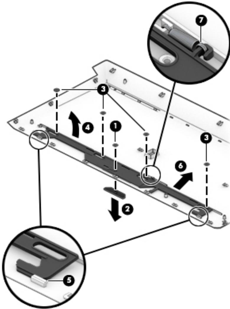
Reverse this procedure to install the service door latch.
