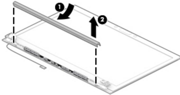
When installing the hinge cover, make sure all cables are routed correctly under the hinge cover and the hooks on the end of the cover are aligned correctly with the snaps on the bottom of the display **(1)**. Press the left **(2)**, and then right **(3)** middle sections of the hinge cover until it snaps into place.
