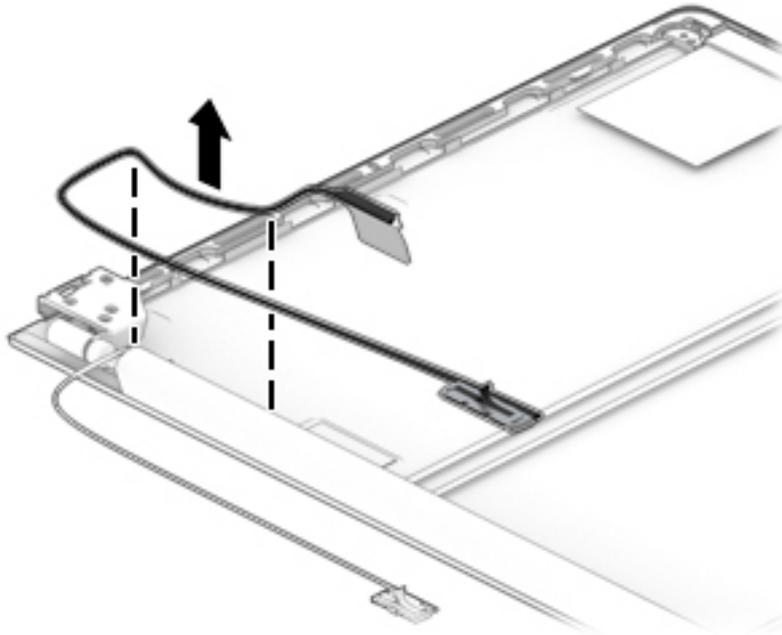
11. If it is necessary to replace the camera/ambient light sensor cable:
