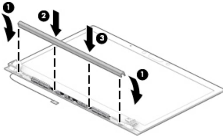
2. To remove the display bezel, flex the top **(1)** of the bezel, the inside edges of the left and right sides **(2)**, and then the bottom **(3)** of the bezel until it disengages from the display enclosure.
