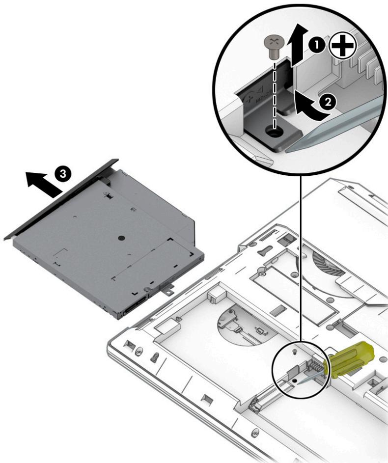
4. To remove the optical drive bracket, remove the two screws (1) securing the bracket to the optical drive, and then remove the bracket (2).
