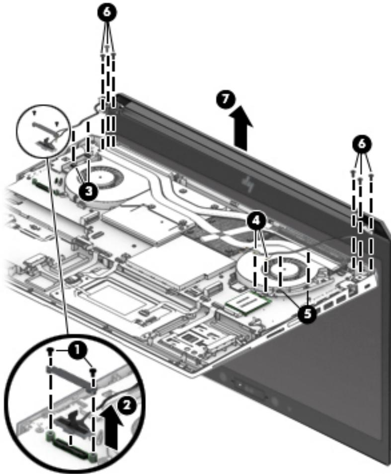
Remove the display assembly components:
