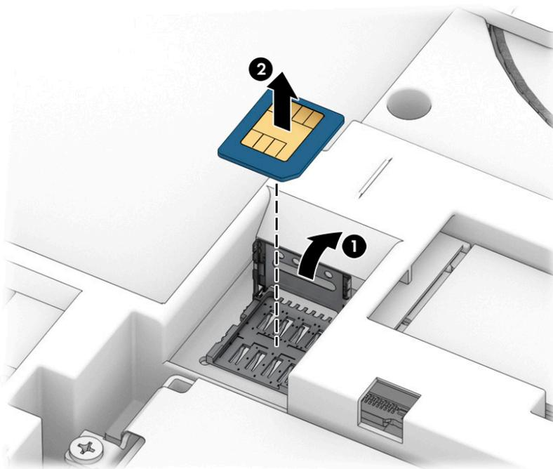
Reverse this procedure to install a SIM card.
