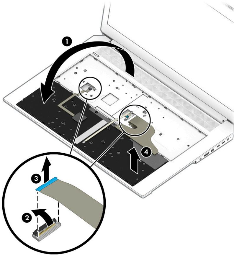
Reverse this procedure to install the keyboard.
