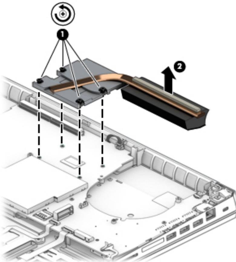
6. Thoroughly clean the thermal material from the surfaces of the heat sink and the system board components each time the heat sink is removed. Thermal paste is used on the processor **(1)** and the heat sink section **(2)** that services it.
