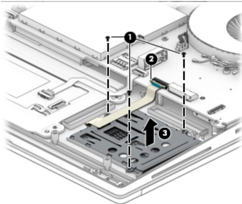
Reverse this procedure to install the smart card board.
