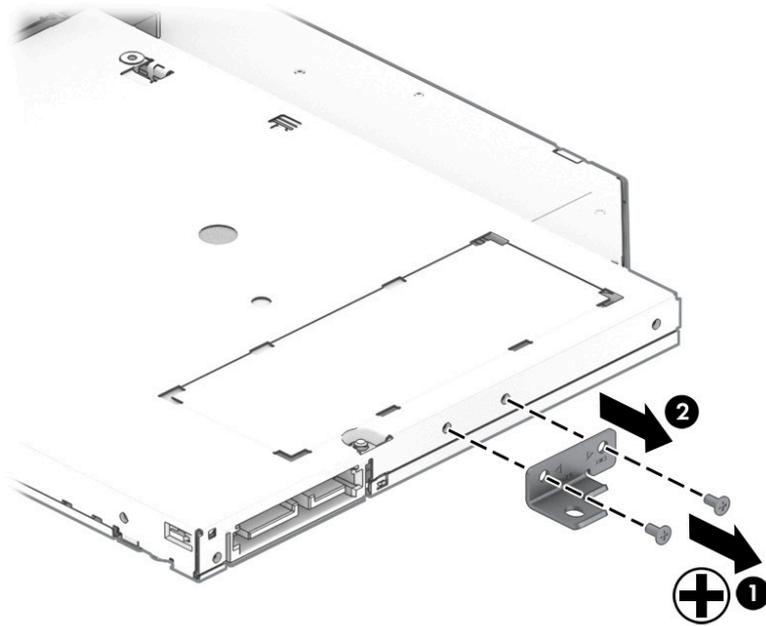
Reverse this procedure to install the optical drive.
