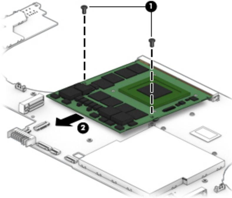
Reverse this procedure to install the discrete MXM graphics card.
