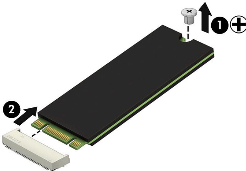
Reverse this procedure to install the solid-state drives.
