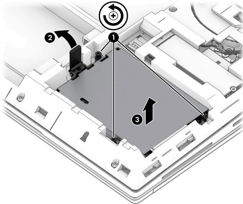
4. If it is necessary to replace the hard drive bracket, remove the four Phillips M3.0 × 3.0 screws **(1)** that secure the bracket to the hard drive, and then lift the bracket straight up **(2)** and remove it from the hard drive.
