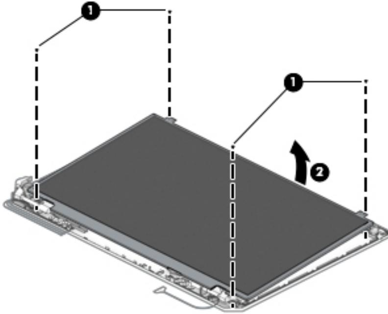
7. Rotate the display panel over onto the keyboard (1).
