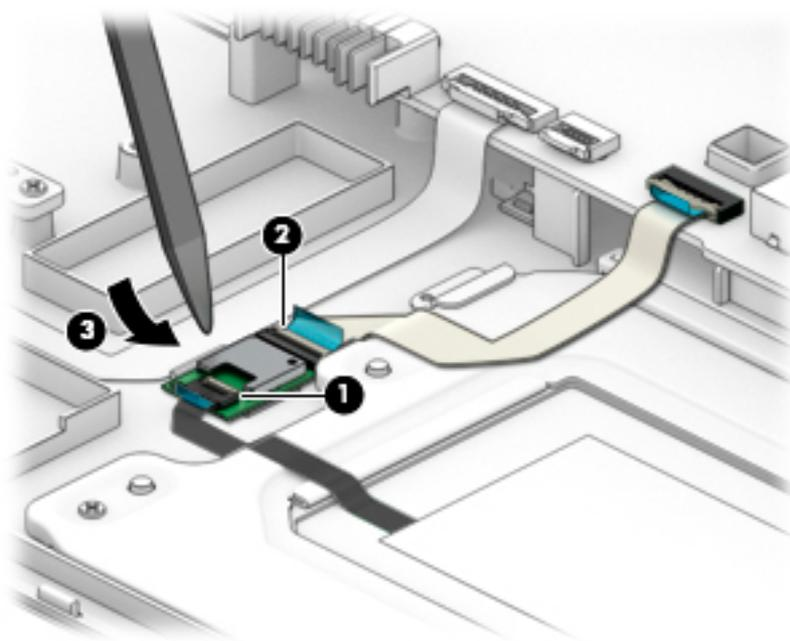
Reverse the removal procedures to install the NFC module.
