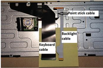
1. Verify whether keyboard flex cables are in good condition (no delamination or torn cable end, no missing or cracked tracks, pads).
