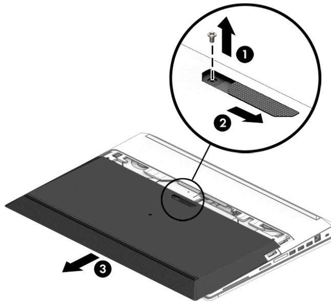
Reverse the removal procedures to install the service door.
