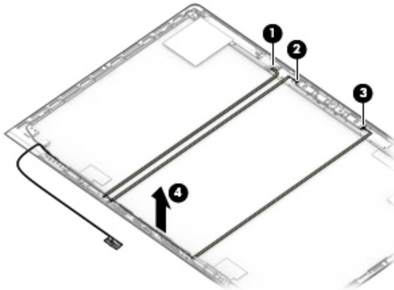
12. If it is necessary to replace the WLAN antenna cables, peel the antennas from the top of the display enclosure (1), remove the antenna cables from the routing path on the bottom of the display enclosure (2), and then remove the antenna cables (3).
