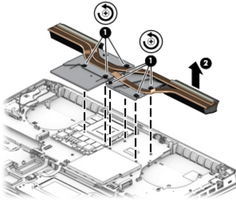
3. Thoroughly clean the thermal material from the surfaces of the heat sink and the system board components each time the heat sink is removed. Thermal paste is used on the processor and graphics processor system board components **(1) (4)** and the heat sink sections **(2) (3)** that service them.
