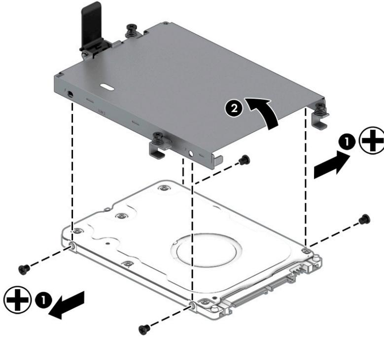
Reverse this procedure to install the hard drive.
