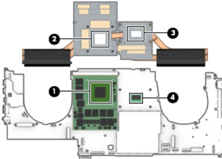
4. **Models with UMA graphics:** Loosen the four captive Phillips screws **(1)** that secure the heat sink to the system board in the order stamped on the heatsink.
