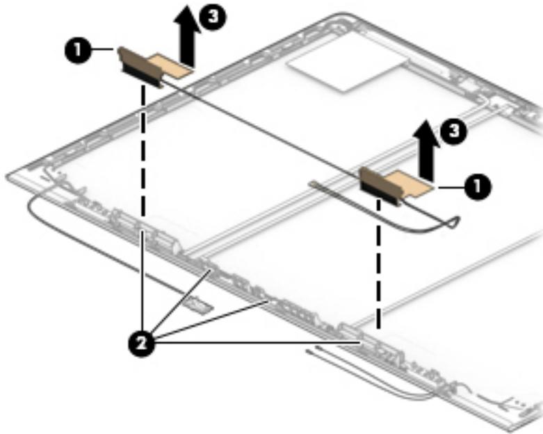
13. If it is necessary to replace the WWAN antenna cables, peel the antennas from the top of the display enclosure (1), remove the antenna cables from the bottom and sides of the display enclosure (2), and then remove the antenna cables (3).
