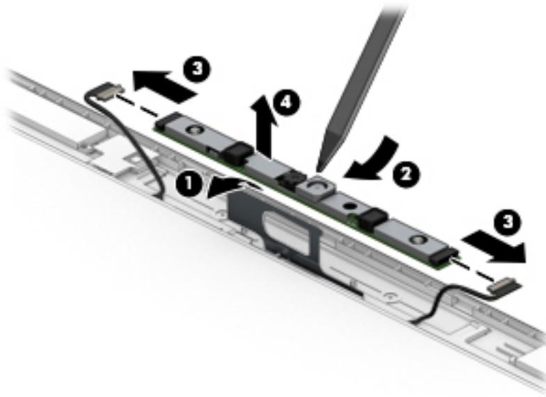
5. If it is necessary to remove the ambient light sensor board, disconnect the cable from the board (1), lift upward to disengage the board from the adhesive on the display enclosure (2), and then remove the board from the display (3).
