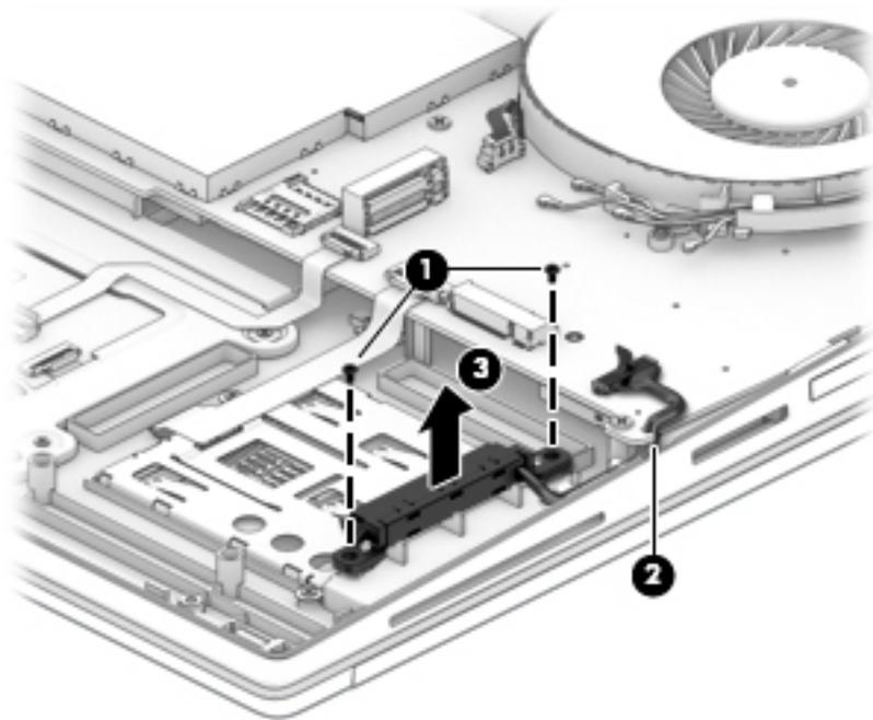
Reverse this procedure to install the hard drive connector.
