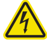
Electric shock hazard
