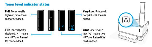
Toner can be added when the **Reload Status** light . next to the reload port glows white. Toner cannot be added when the light is off. To learn how to add toner, follow the instructions on the HP Toner Reload Kit or download the User Guide from www.hp.com/support/Neverstop1000.
