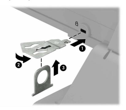
5. Slide the security cable through the security guide installed on the monitor.
