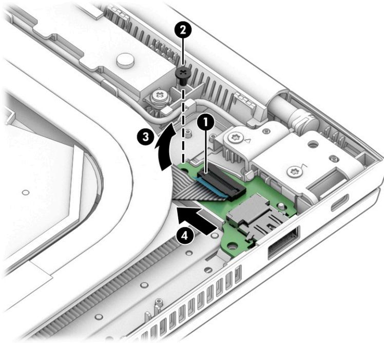
Reverse this procedure to install the USB board.
