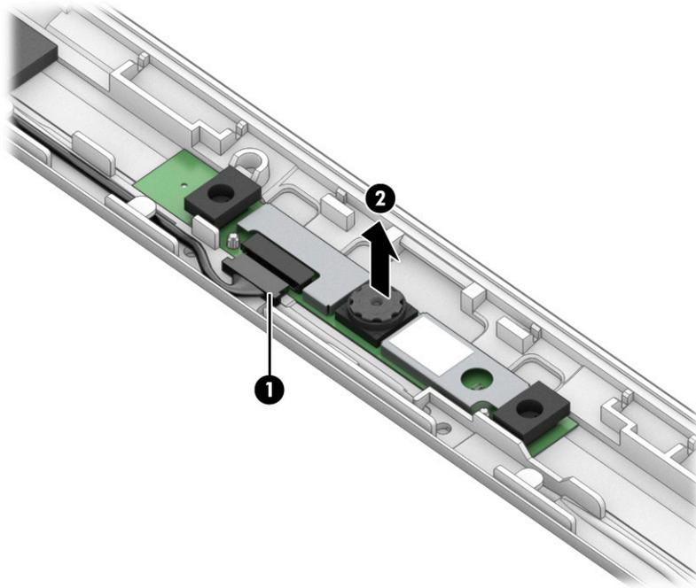
10. If it is necessary to remove or replace the IR camera, disconnect the cable from both sides of the camera **(1)**, and then peel the camera module up to remove it from the adhesive that secures it to the enclosure **(2)**.
