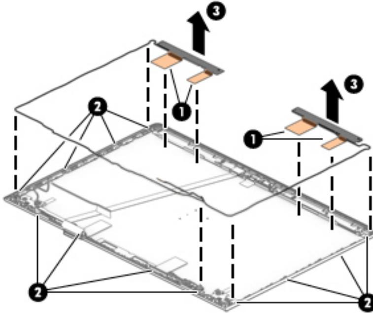
16. If it is necessary to remove or replace the display/camera cable, use the following steps:
