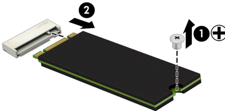
Reverse this procedure to install the solid-state drive.
