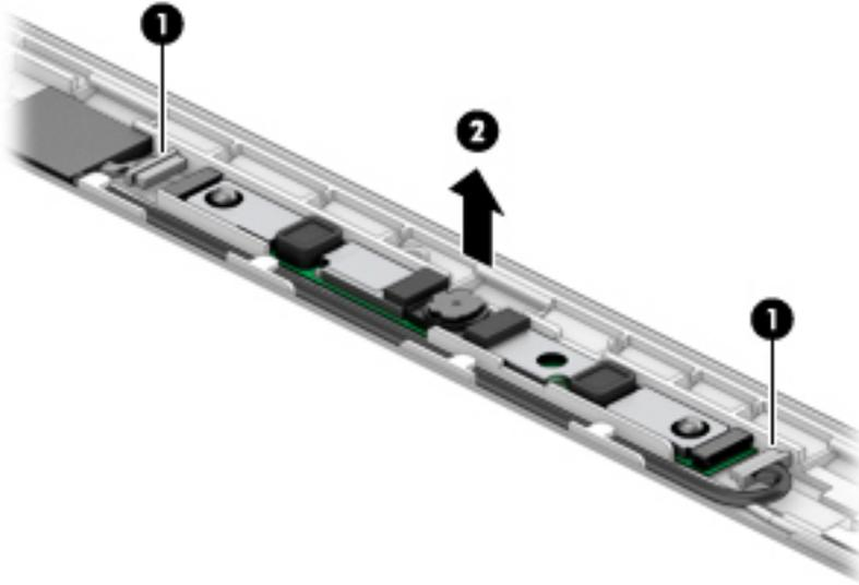
11. If it is necessary to remove the camera privacy cover, lift the cover straight up and off the display.
