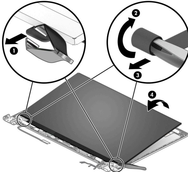
6. Lift the tape from the connector on the display panel (1), lift the locking lever (2), and then disconnect the cable from the panel (3).
