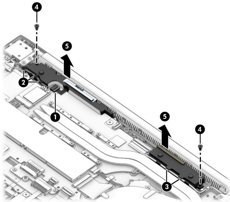
Reverse this procedure to install the speaker assembly.
