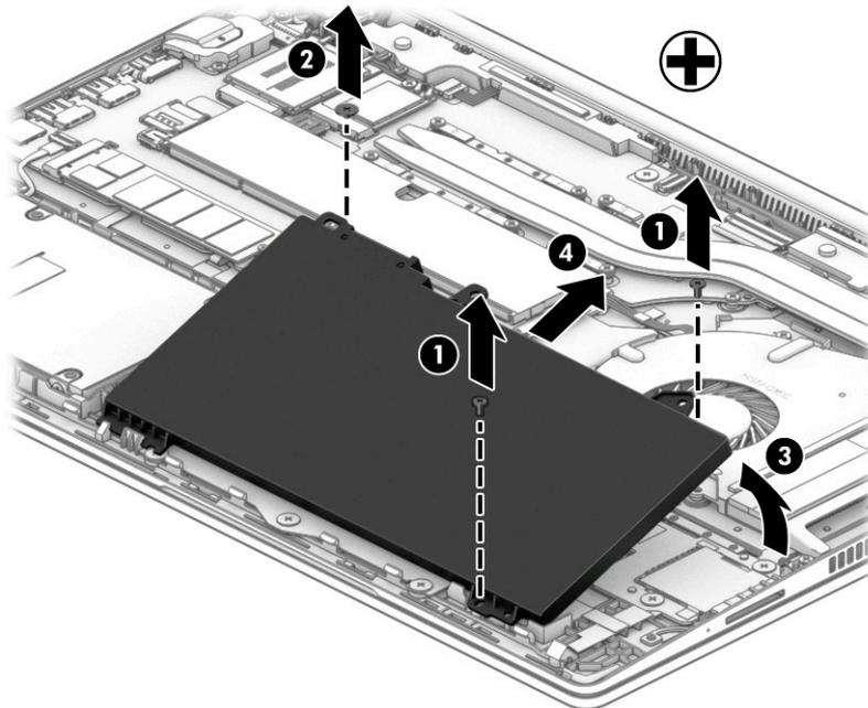
Reverse this procedure to install the battery.
