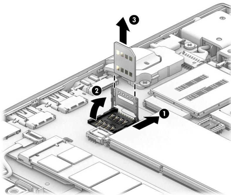
Reverse this procedure to install the SIM card.
