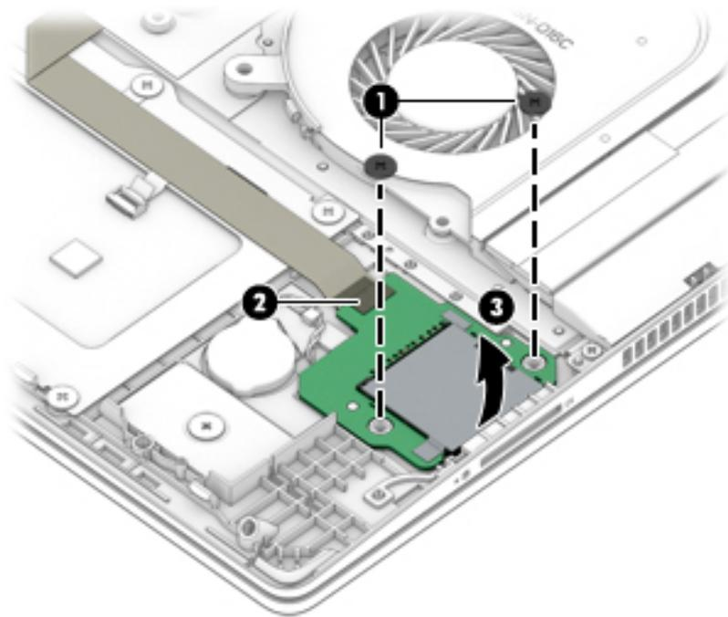
4. Disconnect the RTC battery from the card reader board **(1)**.
