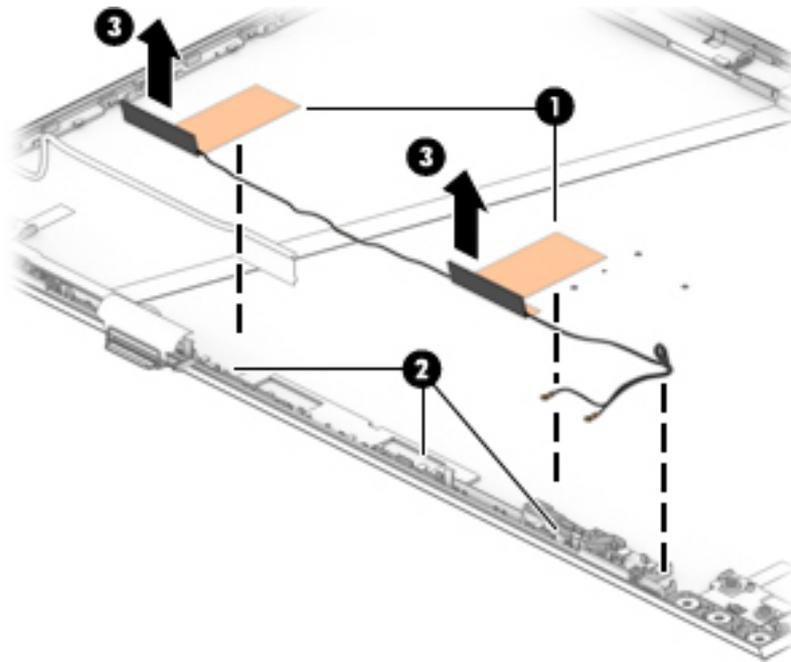
15. If it is necessary to replace the WWAN antennas, peel antennas from the enclosure (1), remove the cables from the clips in the sides of the enclosure (2), and then remove the antennas and cables from the enclosure (3).
