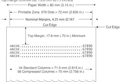
**Note:** The application centers 44 standard character cells ( $13 \times 24$  dots), or 56 compressed character cells ( $10 \times 24$  dots), or 576 addressable bits of graphics across an 80 mm wide receipt. Minimum print line height is 24 dots for text or graphics. Standard print line spacing is 27 dots (that is, 3 extra row dots).
