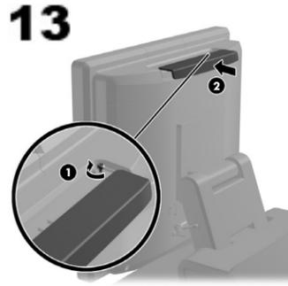
**NOTE:** Tightening the security screw is optional.
