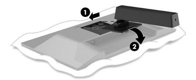
The latch on the bottom of the mounting plate pops up when the stand is locked in place.
