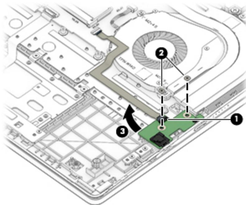
Reverse this procedure to install the power button/audio board.
