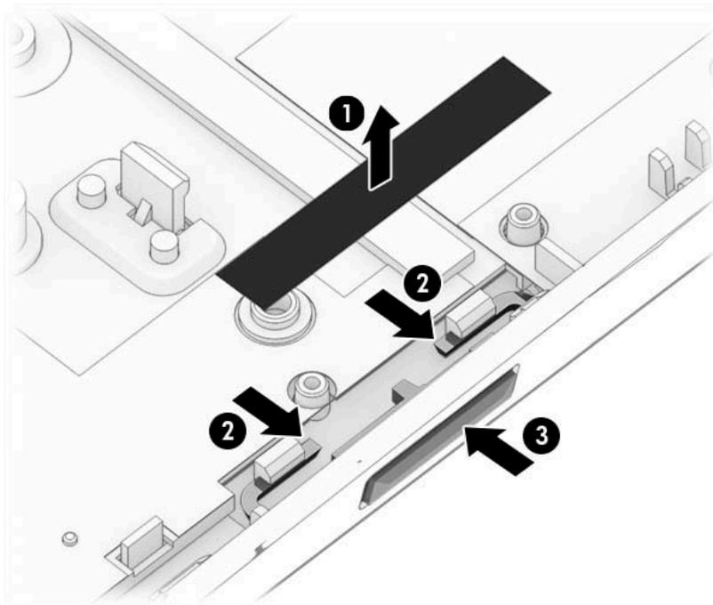
Reverse this procedure to install the power button.
