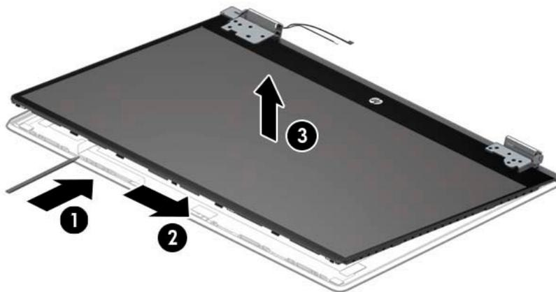
10. If it is necessary to replace the display cable from the display panel:
