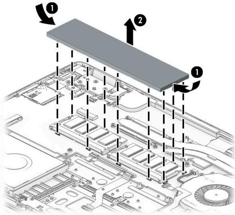
2. Spread the two retention clips outward (1) until the memory module tilts up at a 45-degree angle.
