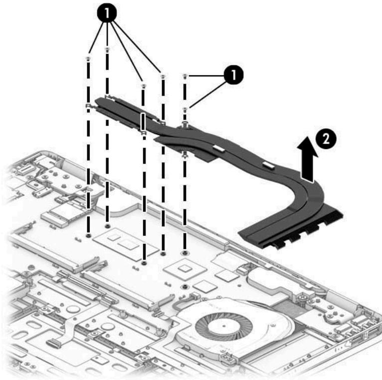
3. Clean and reapply thermal material from the surfaces of the system board components **(1) (3)** and the heat sink **(2) (4)** each time the heat sink is removed.
