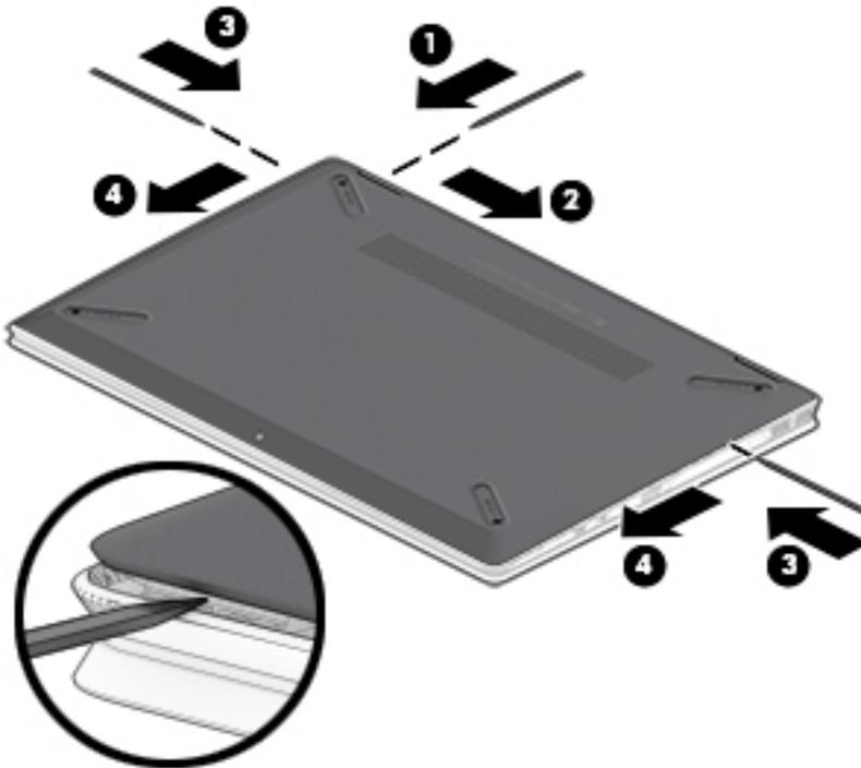
5. On the bottom edge of the computer, insert a plastic tool between the bottom cover and the computer **(1)**, and then slide the tool from one side of the computer to the other **(2)** to separate the bottom cover from the computer. At the same time, push downward on the top edge of the bottom cover **(3)**, and then lift the bottom cover off the computer **(4)**.
