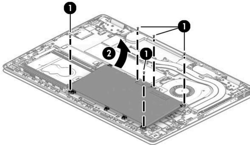
Reverse this procedure to install the battery.
