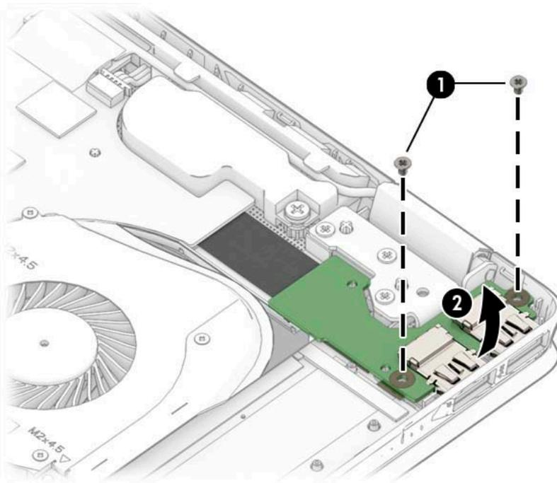
3. Disconnect the cable from the ZIF connector on the USB board **(1)**.
