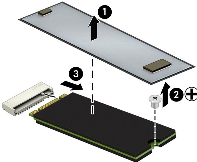
Reverse this procedure to install the solid-state drive.
