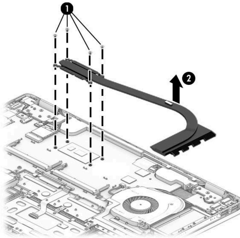
3. Clean and reapply thermal material from the surfaces of the system board component **(1)** and the heat sink **(2)** each time the heat sink is removed.
