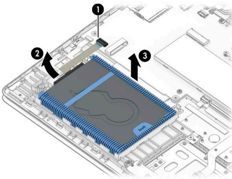
3. If it is necessary to remove the rubber hard drive cover, pull the sides of the cover outward **(1)**, and then remove the cover from the hard drive **(2)**.
