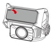
Place and press the bracket firmly onto the electrostatic sticker on the windshield window. Make sure the base is securely locked in place.
