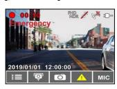
The emergency video recording length is same as the recording interval setting. When the emergency recording length reaches the setting, the system will return to the general recording mode.
