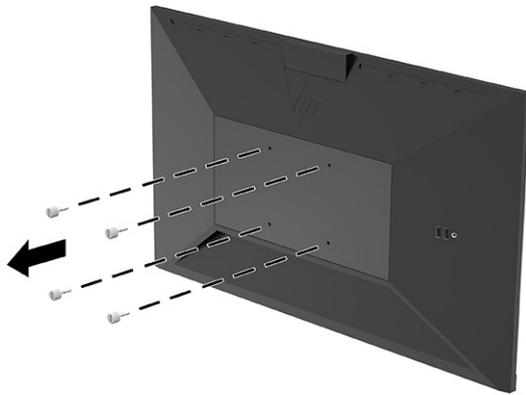
2. To attach the monitor head to a swing arm or other mounting device, insert four mounting screws through the holes on the mounting device and into the VESA screw holes on the back of the monitor head.
