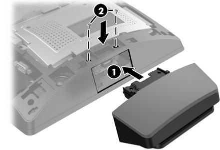
4. Align the tabs on the display head rear cover with the slots on the display head. Place the cover on the display head, and then slide the cover down so that it snaps in place.
