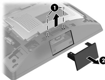
3. Insert the USB connector on the MSR into the side USB port **1**, and then secure the module with the two screws that were previously removed **2**.
