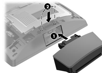
4. Align the tabs on the display head rear cover with the slots on the display head. Place the cover on the display head, and then slide the cover down so that it snaps in place.
