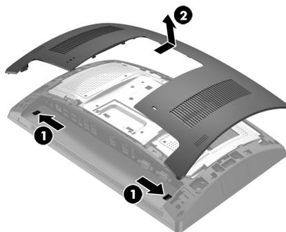
2. Remove the two screws that secure the side port cover **1**, and then pull the port cover off the display head **2**.
