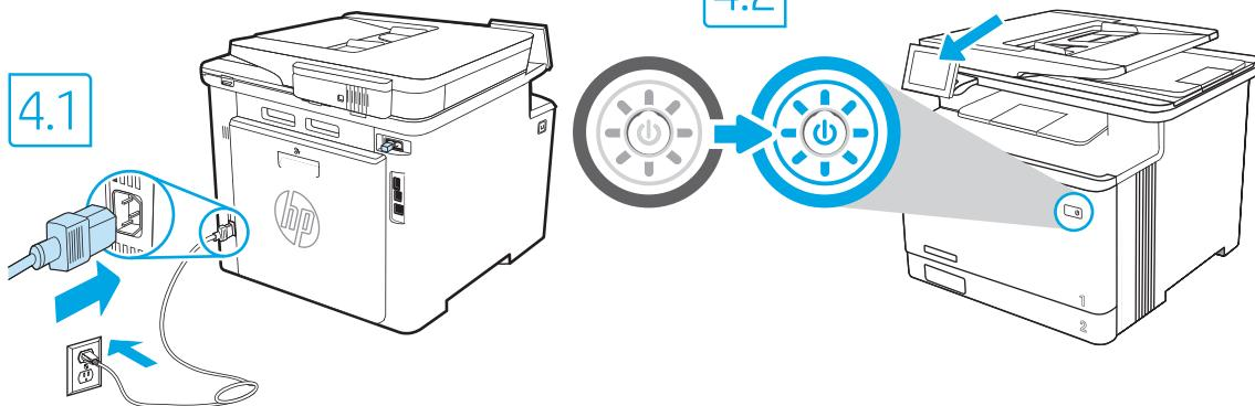
**EN** **4.1** Connect the power cable between the printer and a grounded AC outlet. **4.2** Turn on the printer. **4.3** On the **Initial Setup** screen, set the language, the location, the date/time format, and other features.
