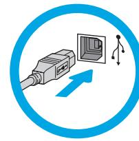
**EN** The USB port is disabled by default and must be enabled from the printer control panel. Open the **Settings** menu, and then select **General, Enable Device USB, Enabled**.
