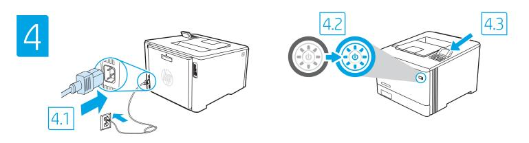
4.1 Connect the power cable between the printer and a grounded AC outlet. 4.2 Turn on the printer. 4.3 On the Initial Setup screen, set the language, the location, the date/time format, and other features.
