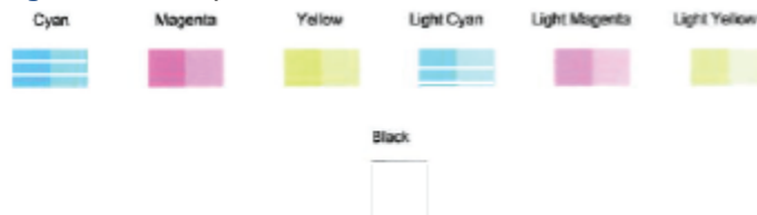
Figure 9-2 Example of color blocks with defects
