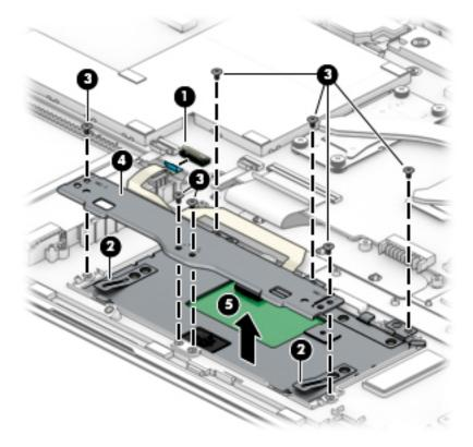
Reverse this procedure to install the TouchPad and bracket.
