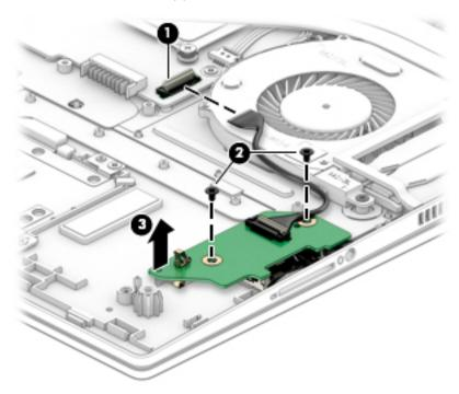
Reverse this procedure to install the SD card board.
