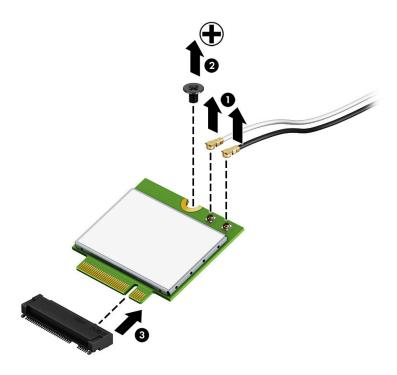
Reverse this procedure to install the WLAN module.
