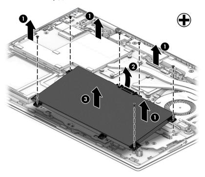
Reverse this procedure to install the battery.
