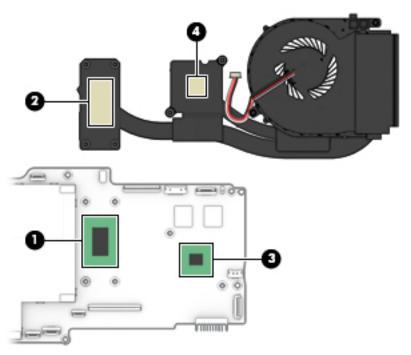
Computer model equipped with a graphics subsystem with UMA memory: Thermal paste is used on the processor (1) and the fan/heat sink assembly section (2) that services it.
