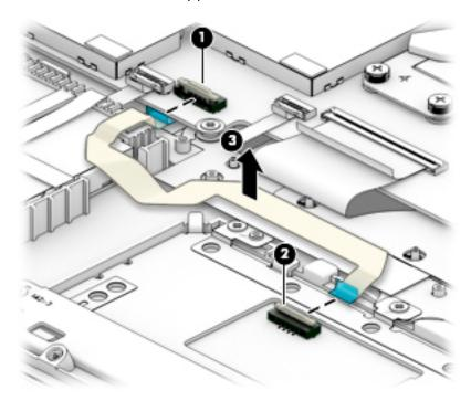
Reverse this procedure to install the TouchPad cable.
