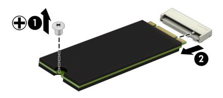
Reverse this procedure to install the solid-state drive.
