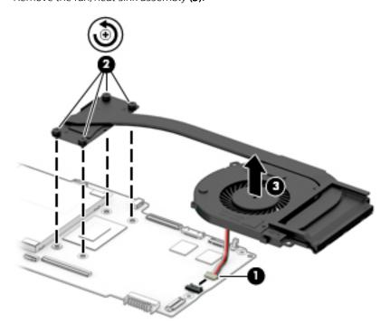
NOTE: The thermal material must be thoroughly cleaned from the surfaces of the fan/heat sink assembly and the system board components each time the fan/heat sink assembly is removed. Replacement thermal material is included with the fan/heat sink assembly and system board spare part kits.
