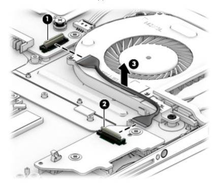
Reverse this procedure to install the SD card board cable.
