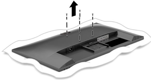
2. To attach the monitor head to a swing arm or other mounting device, insert four mounting screws through the holes on the mounting device and into the VESA screw holes on the back of the monitor head.
