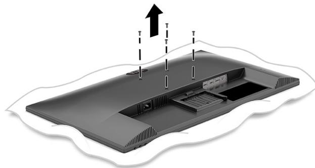
2. To attach the monitor head to a swing arm or other mounting device, insert four mounting screws through the holes on the mounting device and into the VESA screw holes on the back of the monitor head.
